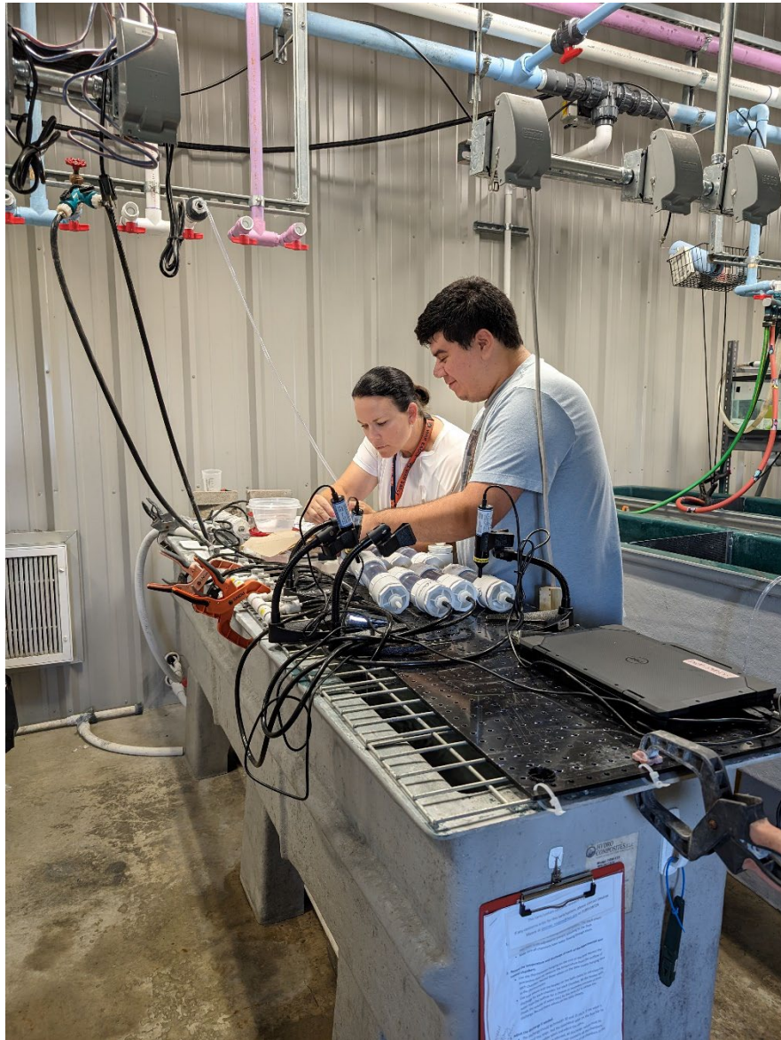
Figure 3. Dr. Shannon Brewer and Brian De La Torre set up the invertebrate tagging trial. Experimental tubes with p-chip scanners are placed on a flow through system. P-chip scanners are placed above the scanning chamber of each experimental tube. Data is automatically collected as tagged beetles move across the scanning chamber.
