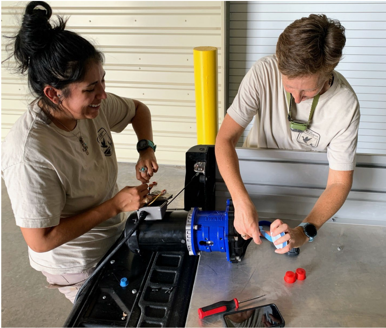
Figure 1. Dominique Alvear (left) and Heidi Meador (right) wiring and preparing a new pump to be replaced on a Refugia tank.
