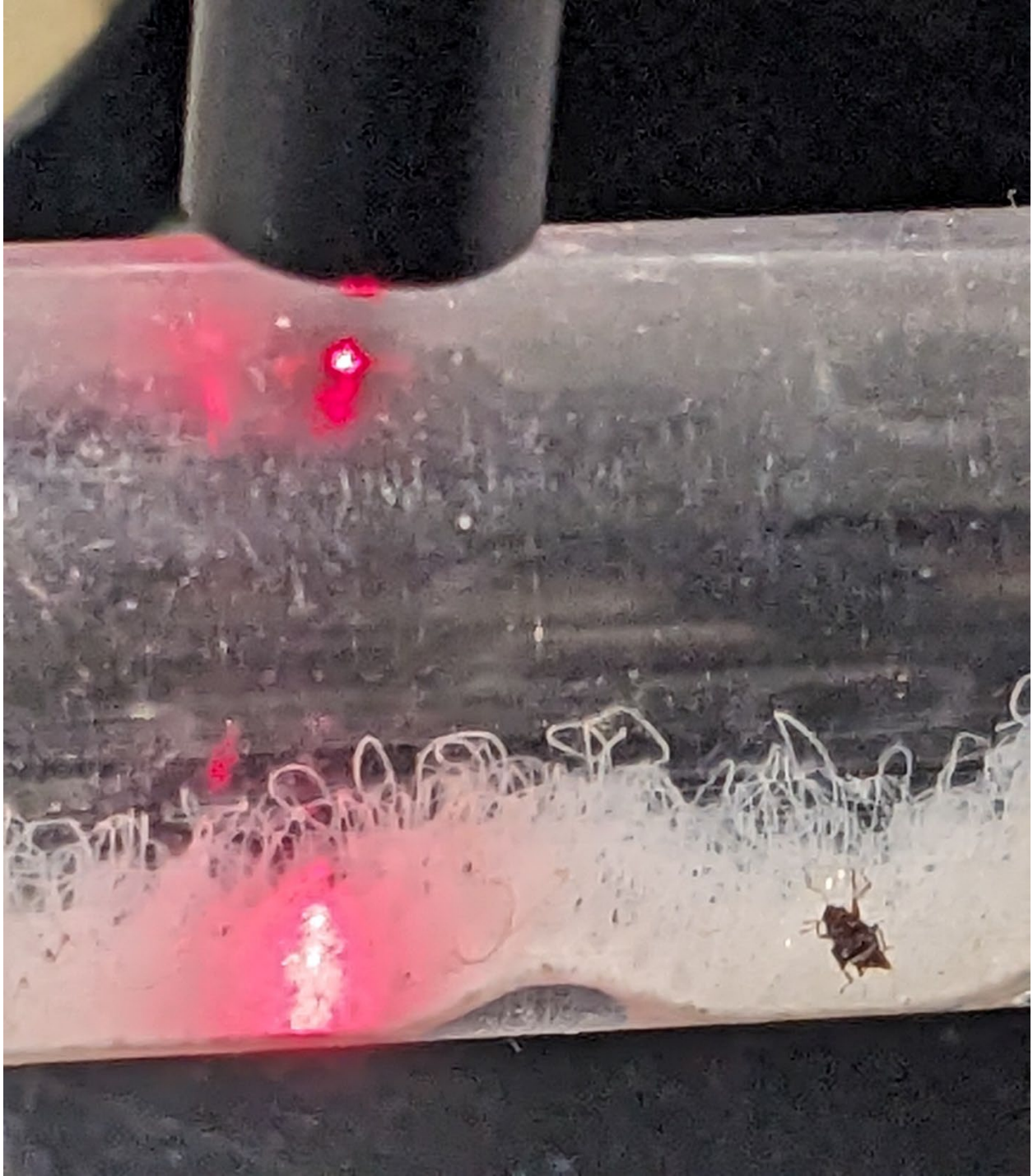
Figure 5. P-Chip tagged beetle on Velcro substrate moving through the scanning tube of the experimental scanning setup.
