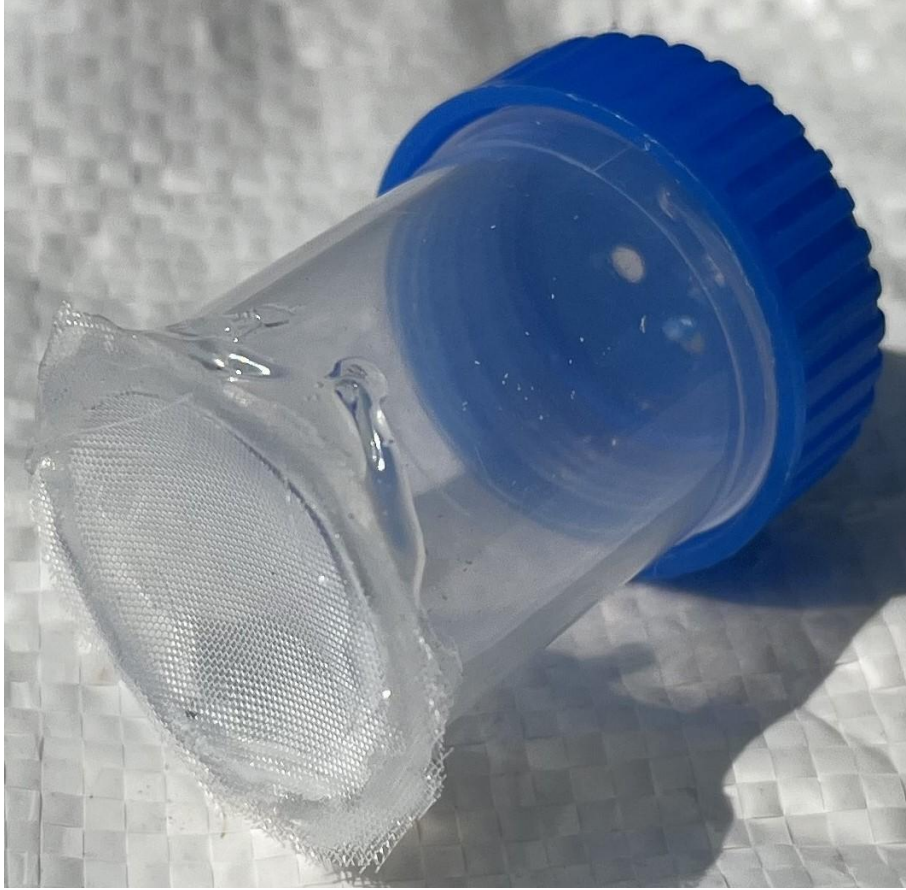
Fig. 2. Photograph of a beetle cage constructed out of polypropylene tubes used for the beetle presence study.
