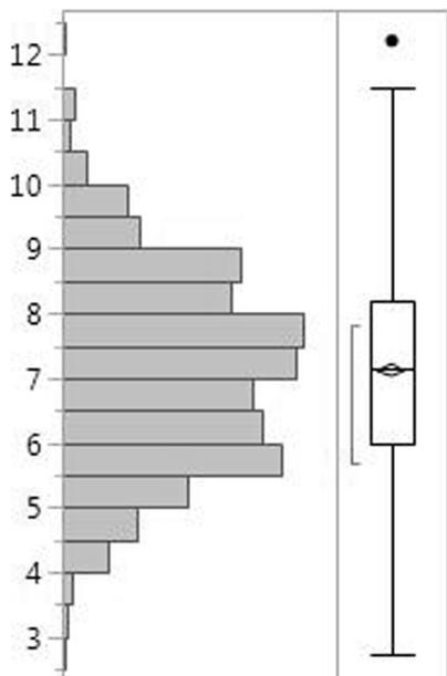
FIGURE 3-3 Range of dissolved oxygen (DO) observed during the drop-net sampling. This shows that DO is less than 4 mg/L at most 2.5 percent of time.  $N = 965$ . No nighttime data are available. SOURCE: Committee manipulation of Edwards Aquifer Authority data.
