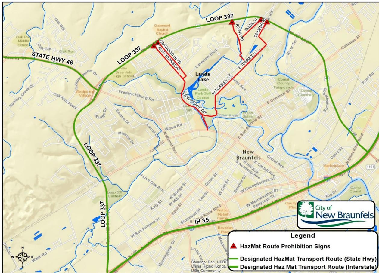
**Figure 3.2-8.** Map of designated HAZMAT transport routes and locations of HAZMAT route prohibition signs.
