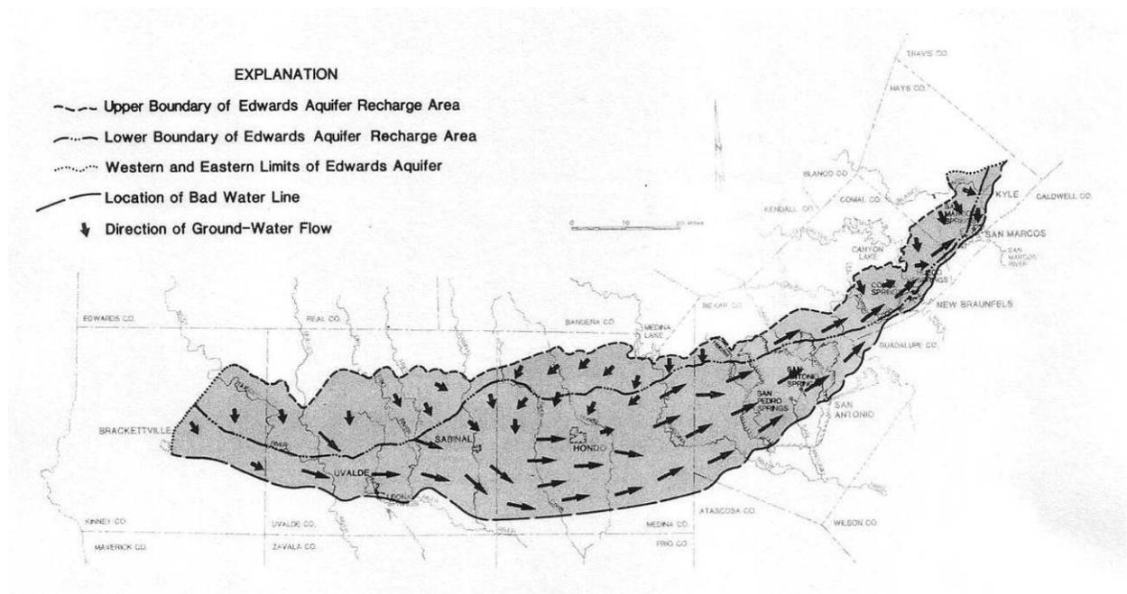
**Figure 4:** General directions of groundwater flow in the Edwards Aquifer between upgradient recharge areas and downgradient discharge areas (from Harden 1988, Figure 9).
