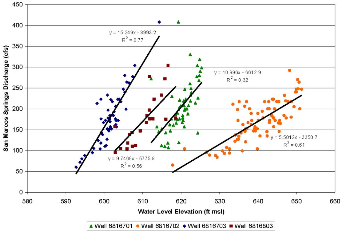
**Figure 13:** Relationship between (1) water level elevations at Well 68-16-701 (Highway 306 Well) located in the Comal Springs Fault Block two miles (three kilometers) east of Hueco Springs and approximately three miles (five kilometers) north-northeast of Comal Springs and wells 68-16-702, 68-16-703, and 68-16-803 and (2) flow at San Marcos Springs (from Johnson and Schindel 2008, Figure 12; cfs = cubic feet per second, ft msl = feet above mean sea level).
