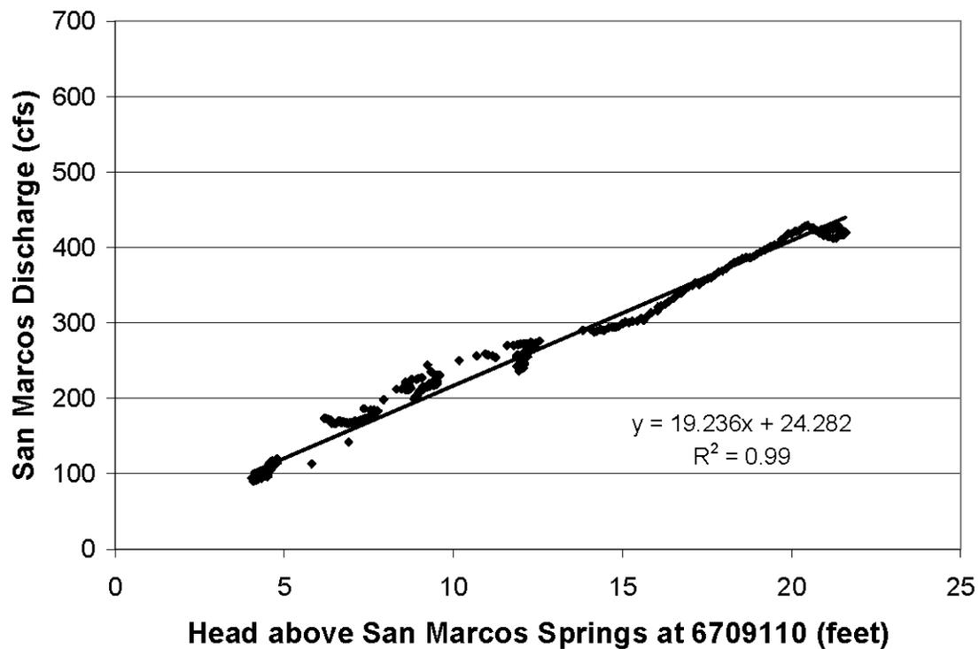
**Figure 12:** Relationship between (1) hydraulic head above San Marcos Springs at Well 67-09-110 (Landa Park or Panther Canyon well) located in the Comal Springs Fault Block five miles (eight kilometers) southwest of San Marcos Springs and (2) flow at San Marcos Springs (from Johnson and Schindel 2008, Figure 38; cfs = cubic feet per second).
