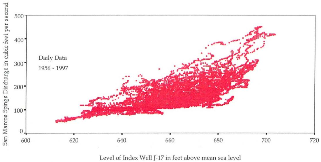
**Figure 10:** Relationship between (1) water level elevations at Index Well J-17 and (2) flow at San Marcos Springs (modified from Votteler 2000, Figure 17).
