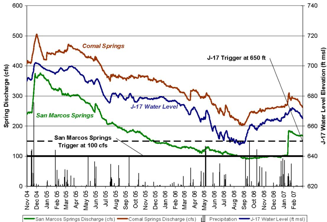
**Figure 1:** Comparison of Index Well J-17 water levels with Comal and San Marcos springflows for the period between November 2004 and February 2007 (from Johnson and Schindel 2008; cfs = cubic feet per second; ft msl = feet above mean sea level).
