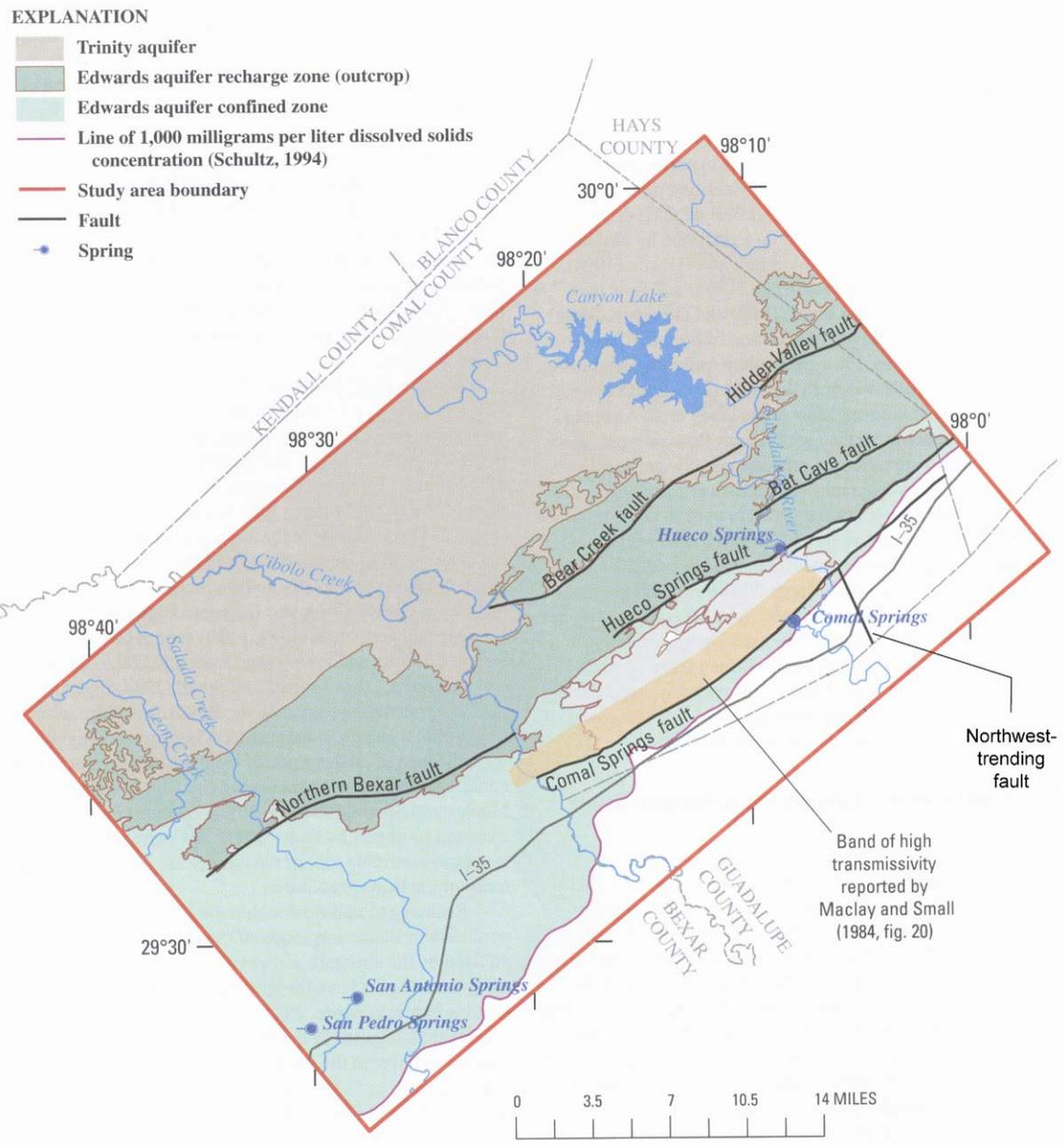
**Figure 5:** Main geologic structural features in the Comal Springs area including a northwest-trending fault located east of Comal Springs (modified from Otero 2007).
