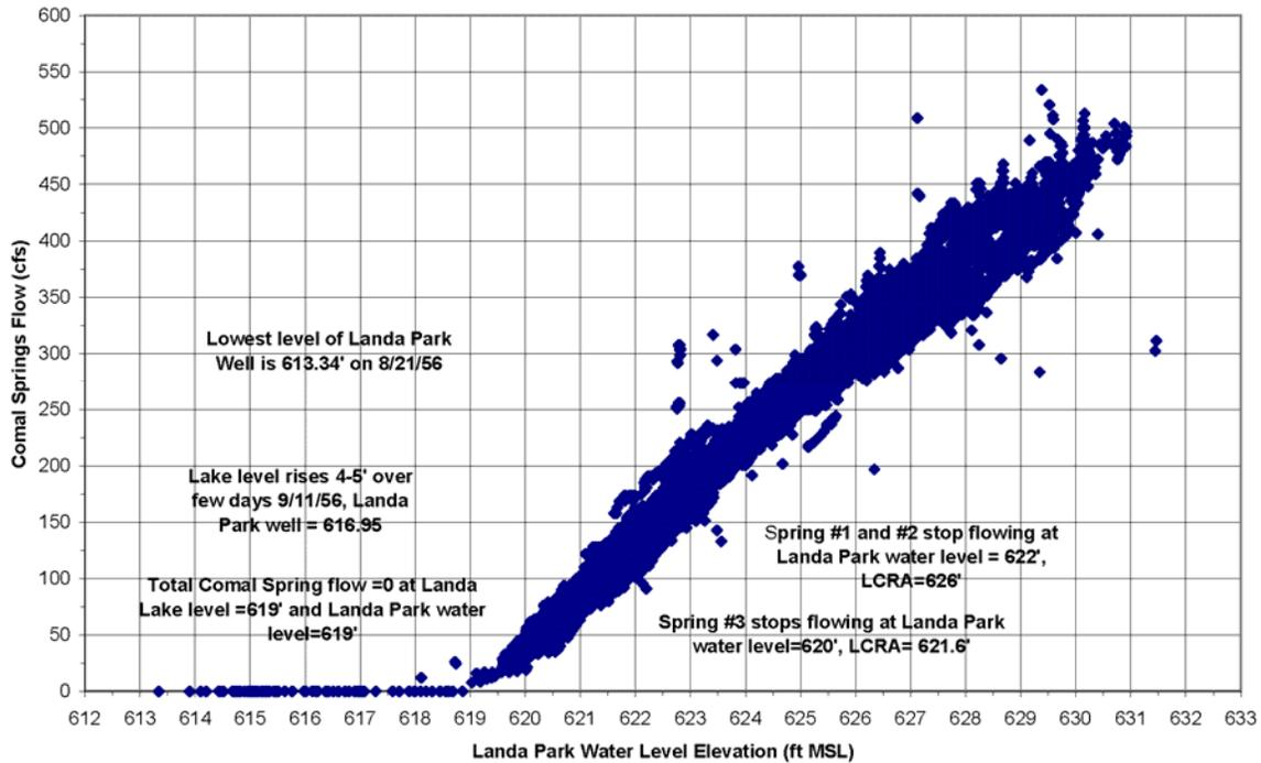
**Figure 11:** Relationship between (1) water level elevation at Well 68-23-302 (Landa Park or Panther Canyon well) located in the Comal Springs Fault Block half a mile (0.8 kilometer) west of Comal Springs and (2) flow at Comal Springs (from LBG-Guyton Associates 2004, Figure B-13; cfs = cubic feet per second, ft MSL = feet above mean sea level, ' = feet, LCRA = reference to a well operated by the Lower Colorado River Authority during the 1950s).
