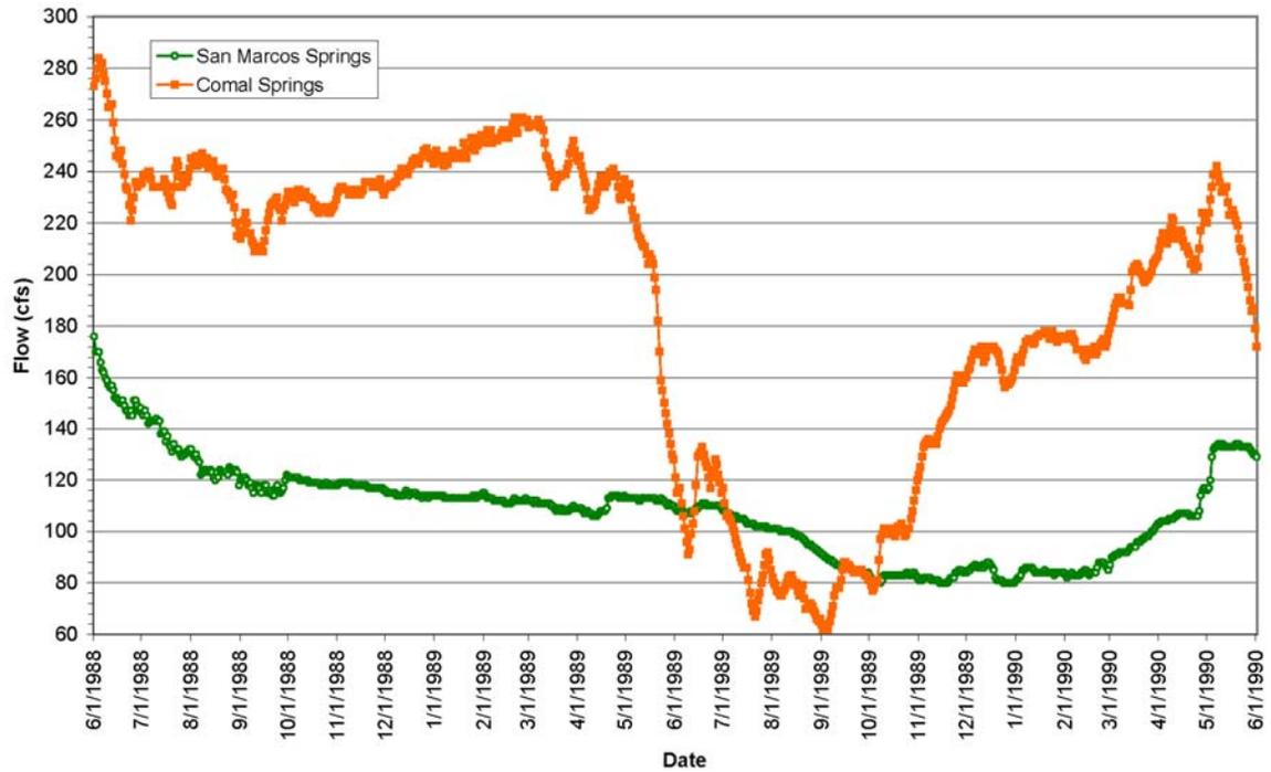
**Figure 14:** Flow at Comal and San Marcos springs for the period of 1988 to 1990 (modified from LBG-Guyton Associates 2004, Figure B-28; cfs = cubic feet per second).
