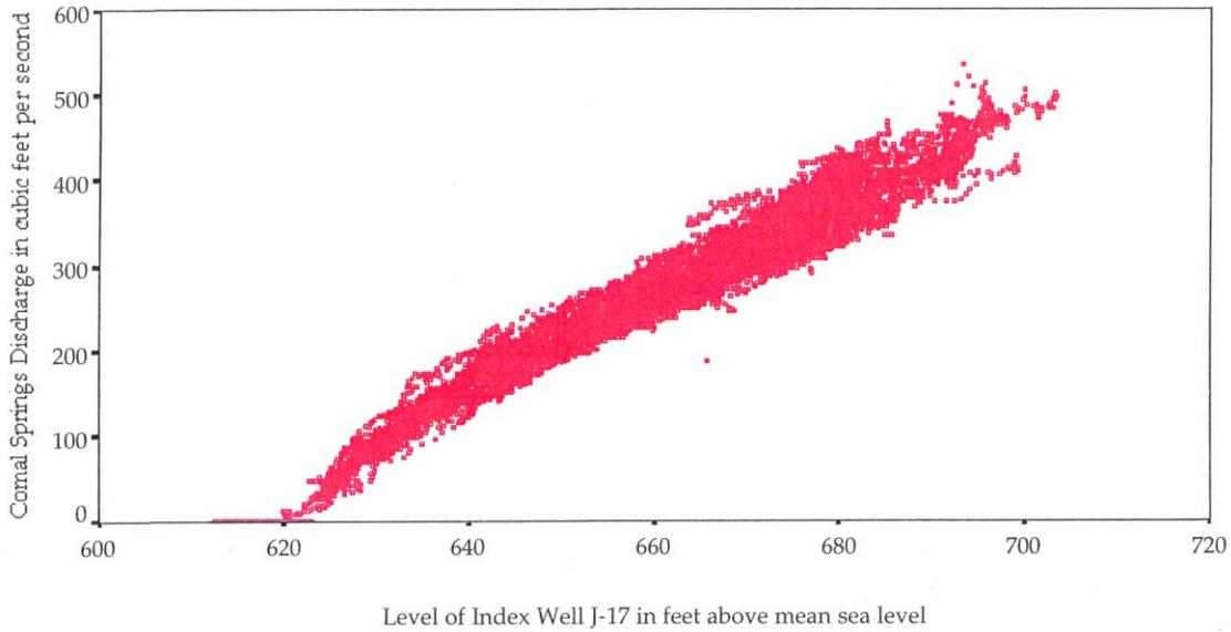
**Figure 9:** Relationship between (1) water level elevation at Index Well J-17 and (2) flow at Comal Springs (modified from Votteler 2000, Figure 14).
