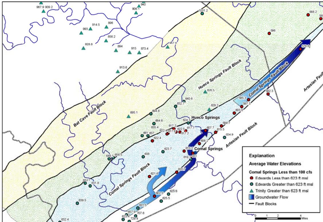
**Figure 6:** Groundwater flow in the Artesian and Comal Springs fault blocks (from Johnson and Schindel 2008; cfs = cubic feet per second; ft msl = feet above mean sea level).
