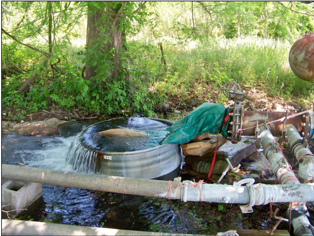
Figure 2. A shade sock secured over a net on the outlet at the Aldridge Corporate well. This net rests in a tub in order to reduce degradation of specimens that can result from battering.
