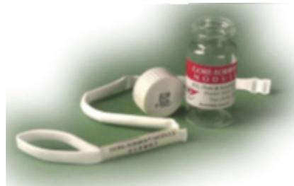
**Figure 5. Universal Passive Sampler and Its Glass Vial (ITRC, 2005)**
