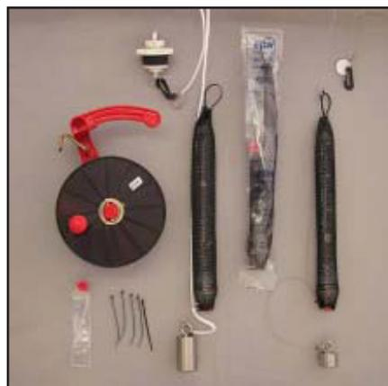
**Figure 3. Polyethylene Diffusion Bag Samplers (ITRC, 2005)**
