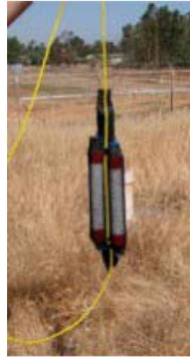
**Figure 4. Rigid Porous Polyethylene Samplers (ITRC, 2005)**
