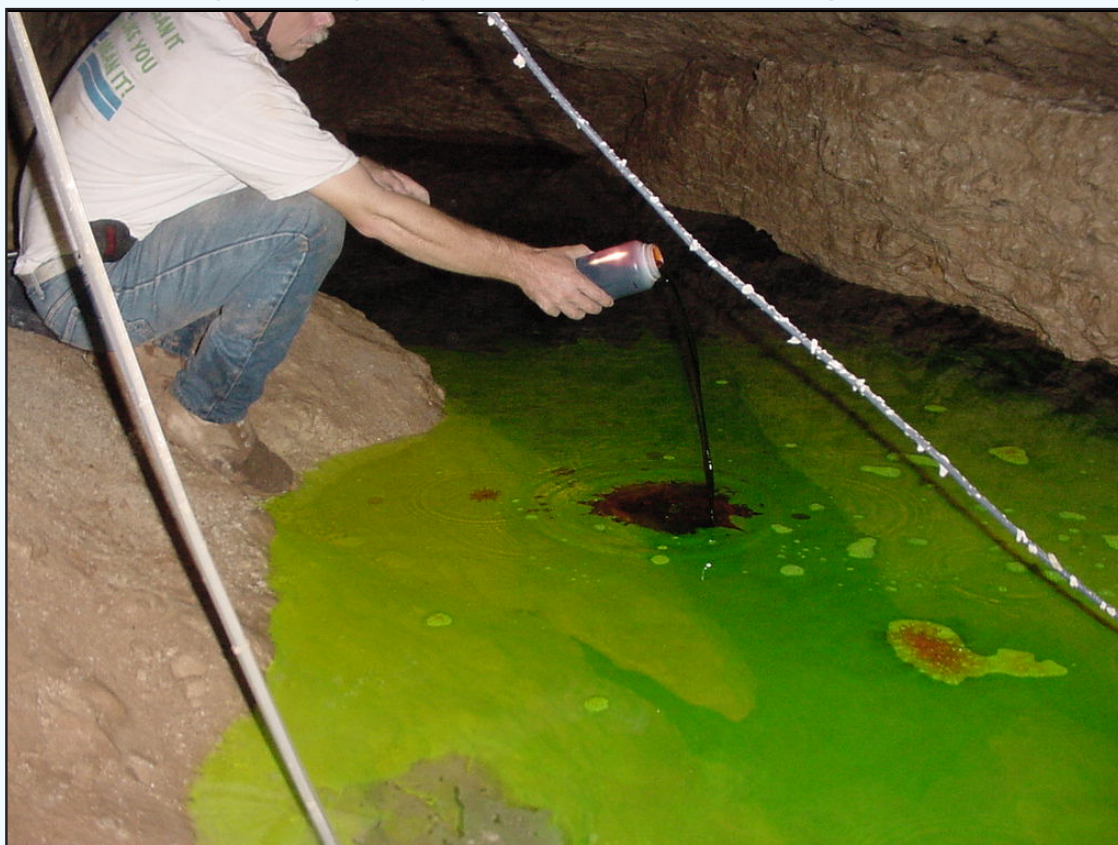
Figure 13. Dye Injection at Ezell's Cave on July 5, 2005
