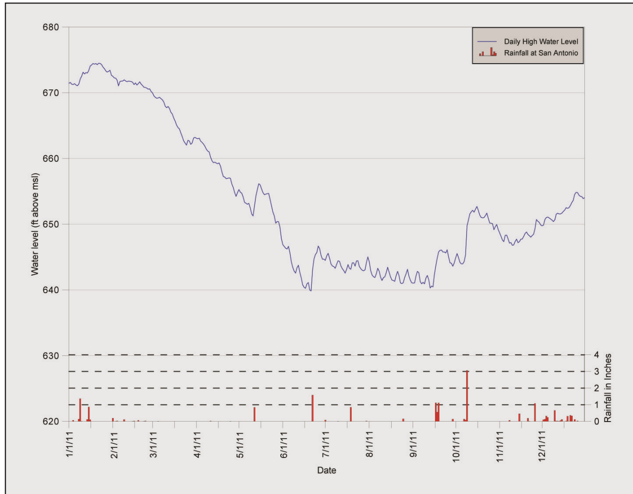
Figure B-1. Bexar County Index Well J-17 (AY-68-37-203) Hydrograph of Groundwater Elevation vs. Precipitation at San Antonio International Airport
