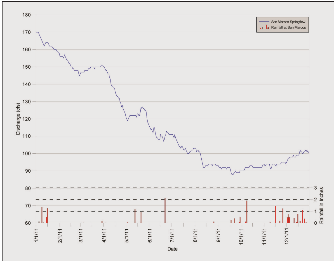
Figure B-5. San Marcos Springflow Hydrograph of Springflow vs. Precipitation at San Marcos
