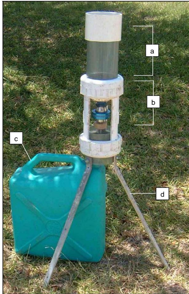
Figure 4. Modified filtration apparatus. a) prefilters (220 $\mu$ m and 86 $\mu$ m). b) sample filter mount with 30  $\mu$ m monofilament filter. c) 22.7 L formalin collection container. d) filter apparatus support.
