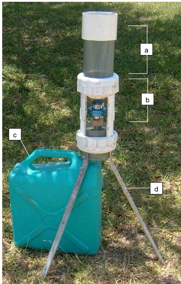
**Figure 2. Modified filtration apparatus. a) prefilters (220  $\mu\text{m}$  and 86  $\mu\text{m}$ ). b) sample filter mount with 30  $\mu\text{m}$  monofilament filter. c) 22.7 L formalin collection container. d) filter apparatus support.**
