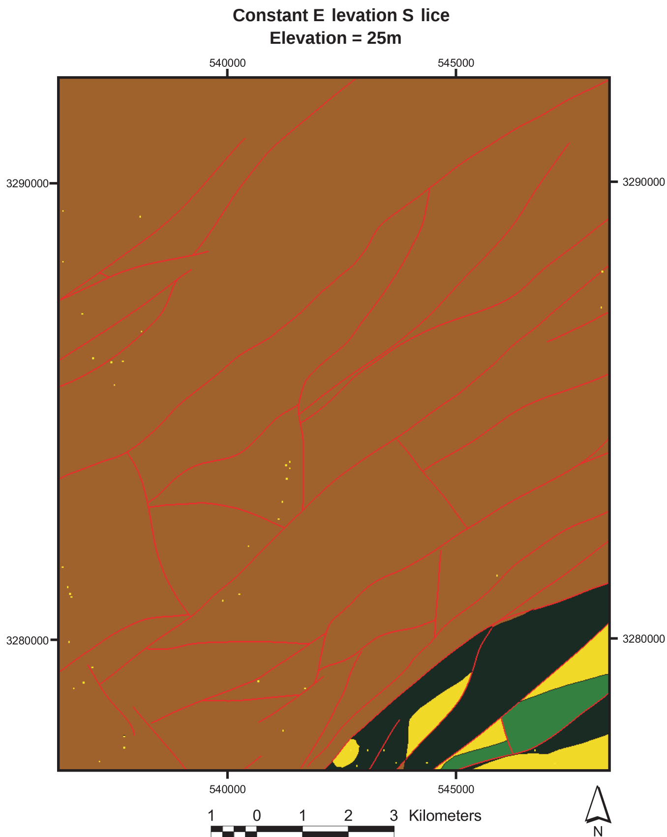
Figure 3-32. Map view of constant elevation (horizontal) slice through model. Elevation = 25 m. Units are UTM meters, NAD27. Red lines show fault traces, and yellow points show well locations. See Figure 3-1 for complete color key.
