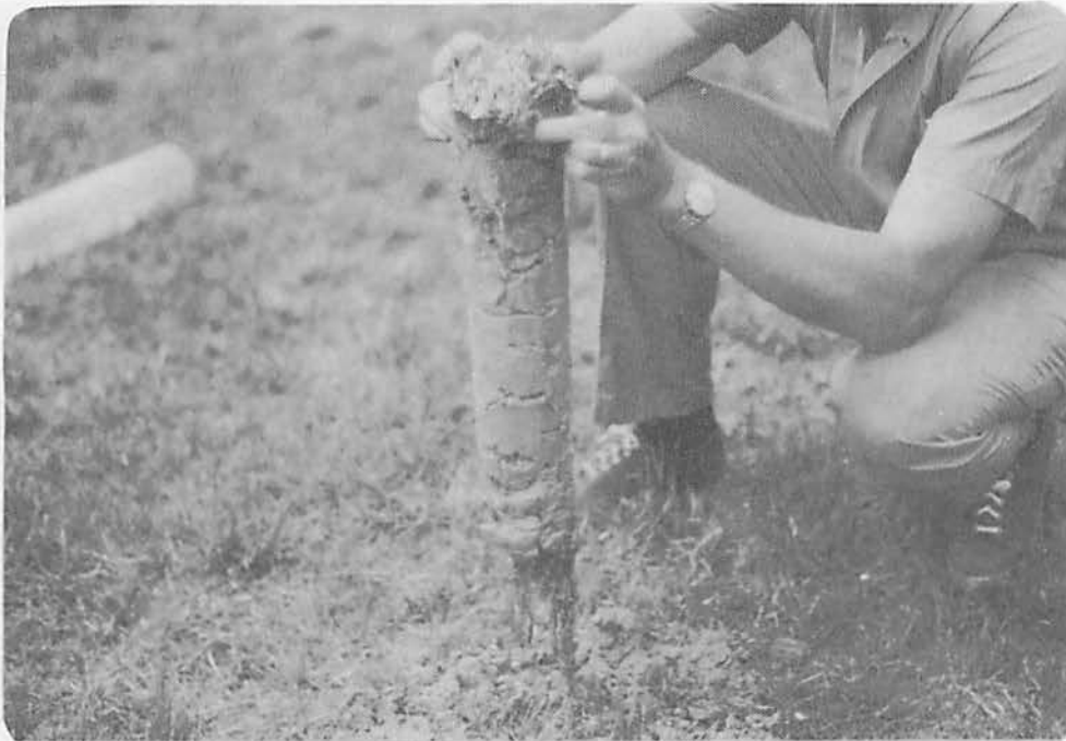
Plug Taken from Tank 10 Showing Extent of Root Penetration by Carpet Grass.
