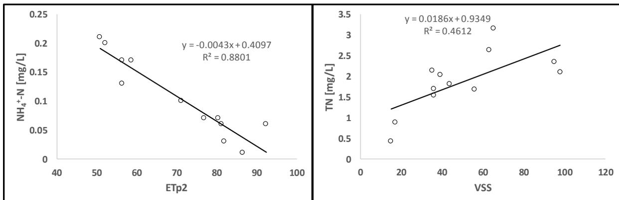
Figure 32. Examples of EMC regression models for TN and  $\text{NH}_4^+\text{-N}$ .
