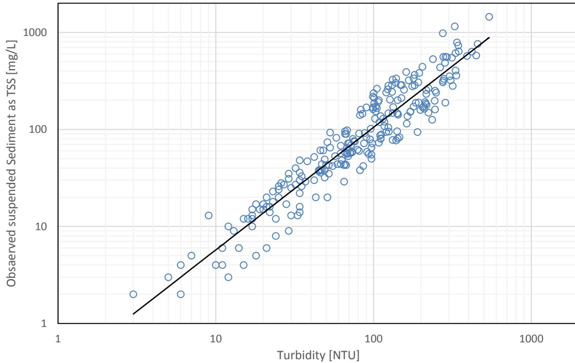
Figure 18. Turbidity vs observed suspended sediment (i.e., TSS) concentrations.
