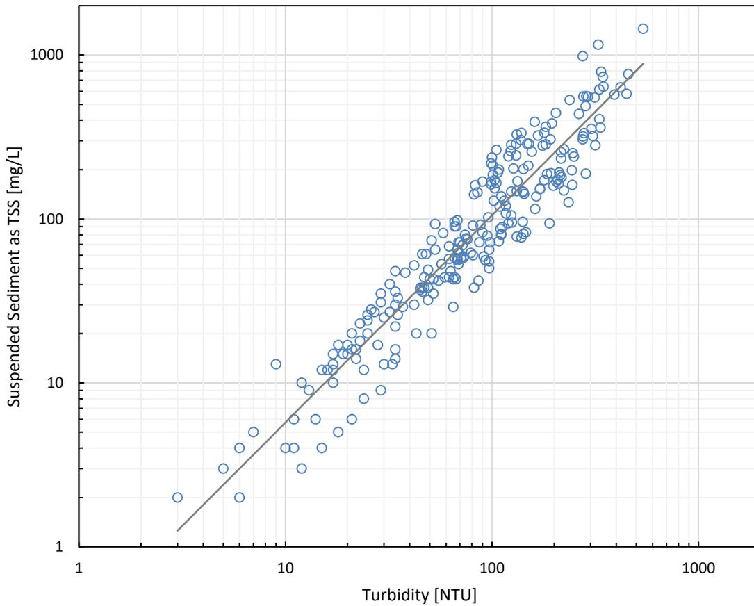
Figure 7. Relationship between turbidity (15-min interval) and suspended sediment measured as total suspended solids (TSS) at Sessom Creek, 27 March to 7 December 2018.
