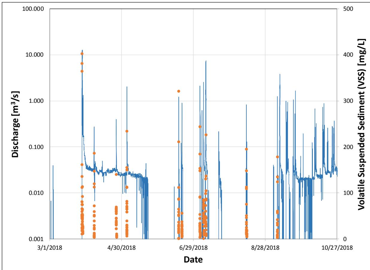
Figure 29. Volatile Suspended Sediments (VSS) concentrations in stormwater samples. VSS is the organic portion of Total Suspended Sediments (TSS). Note that the NPS axis is linear, while the discharge axis is logarithmic.
