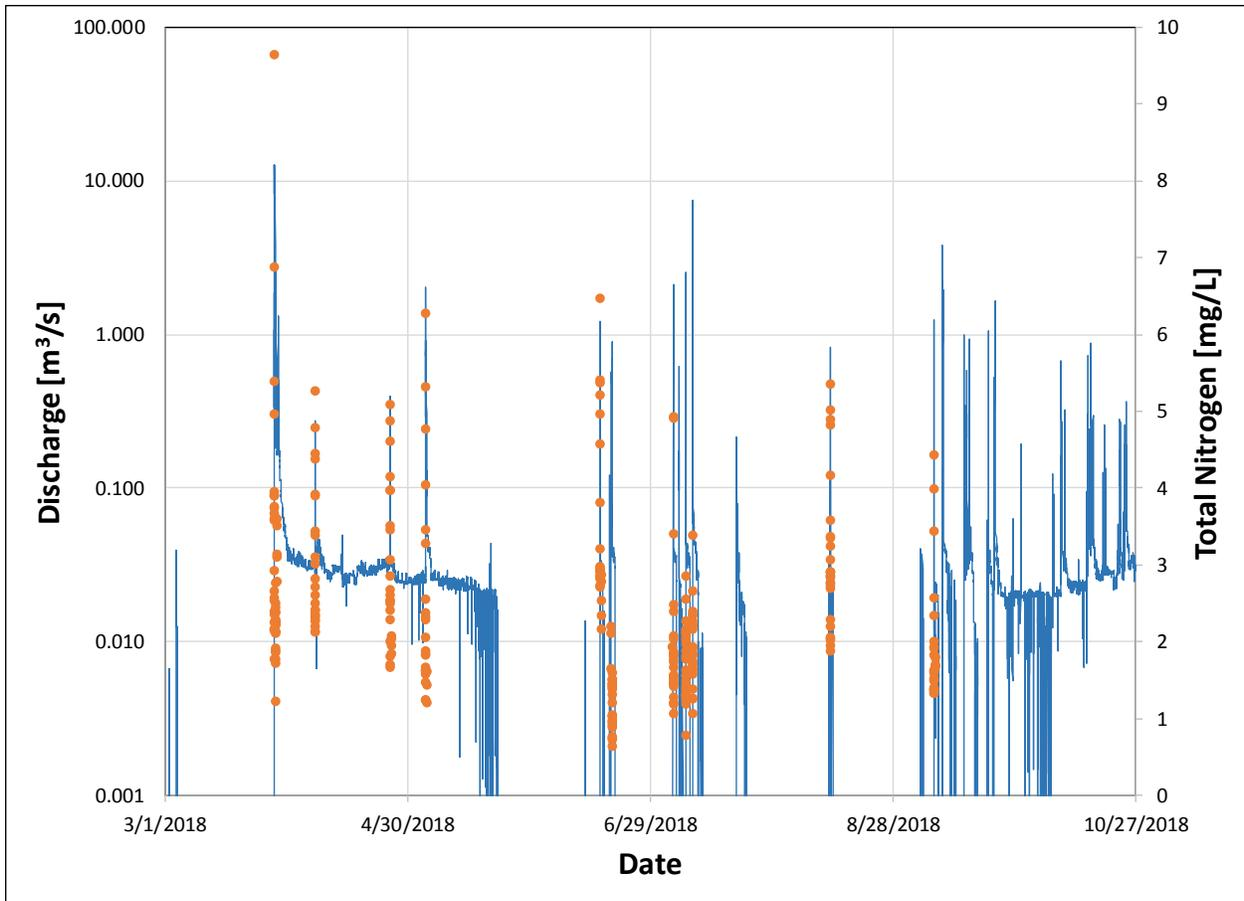
Figure 25. Total Nitrogen concentrations in stormwater samples.
