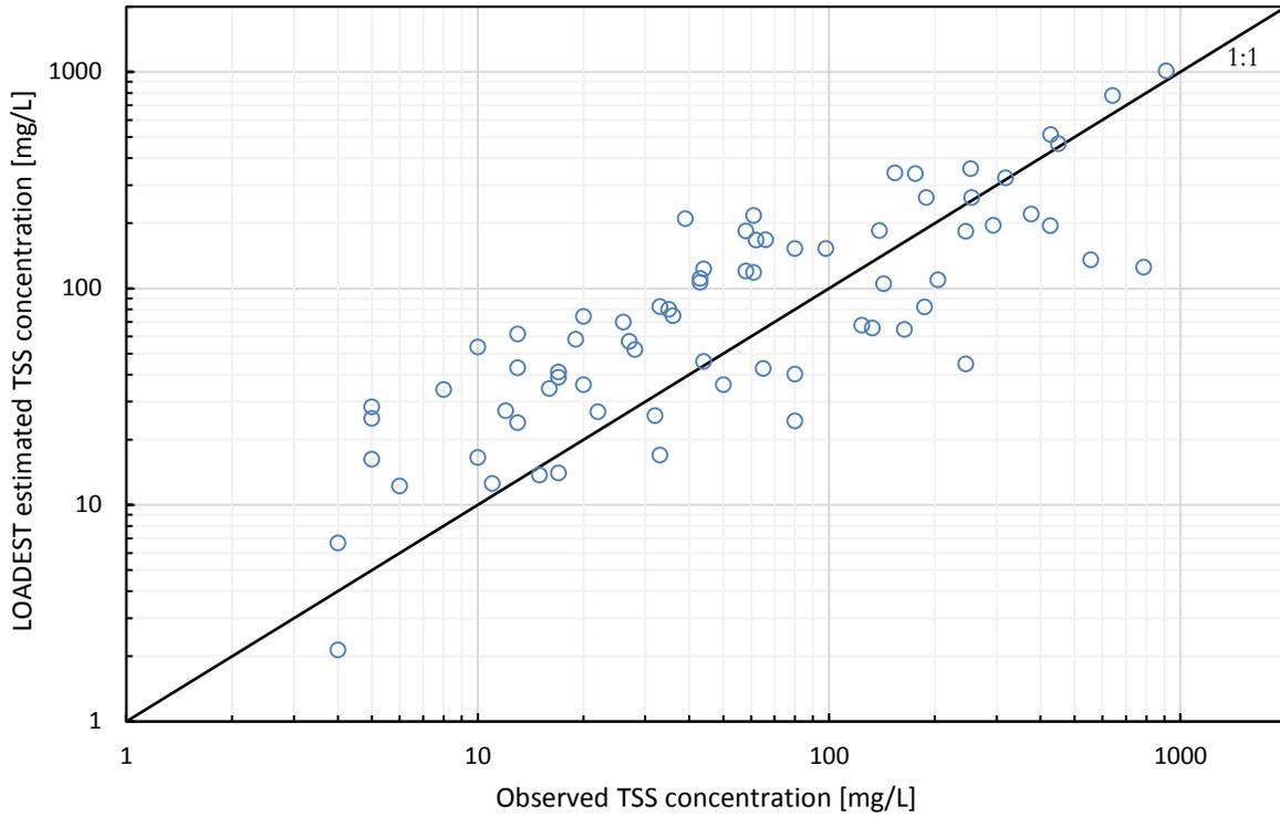
Figure 12. Observed vs LOADEST estimated suspended sediment concentrations.
