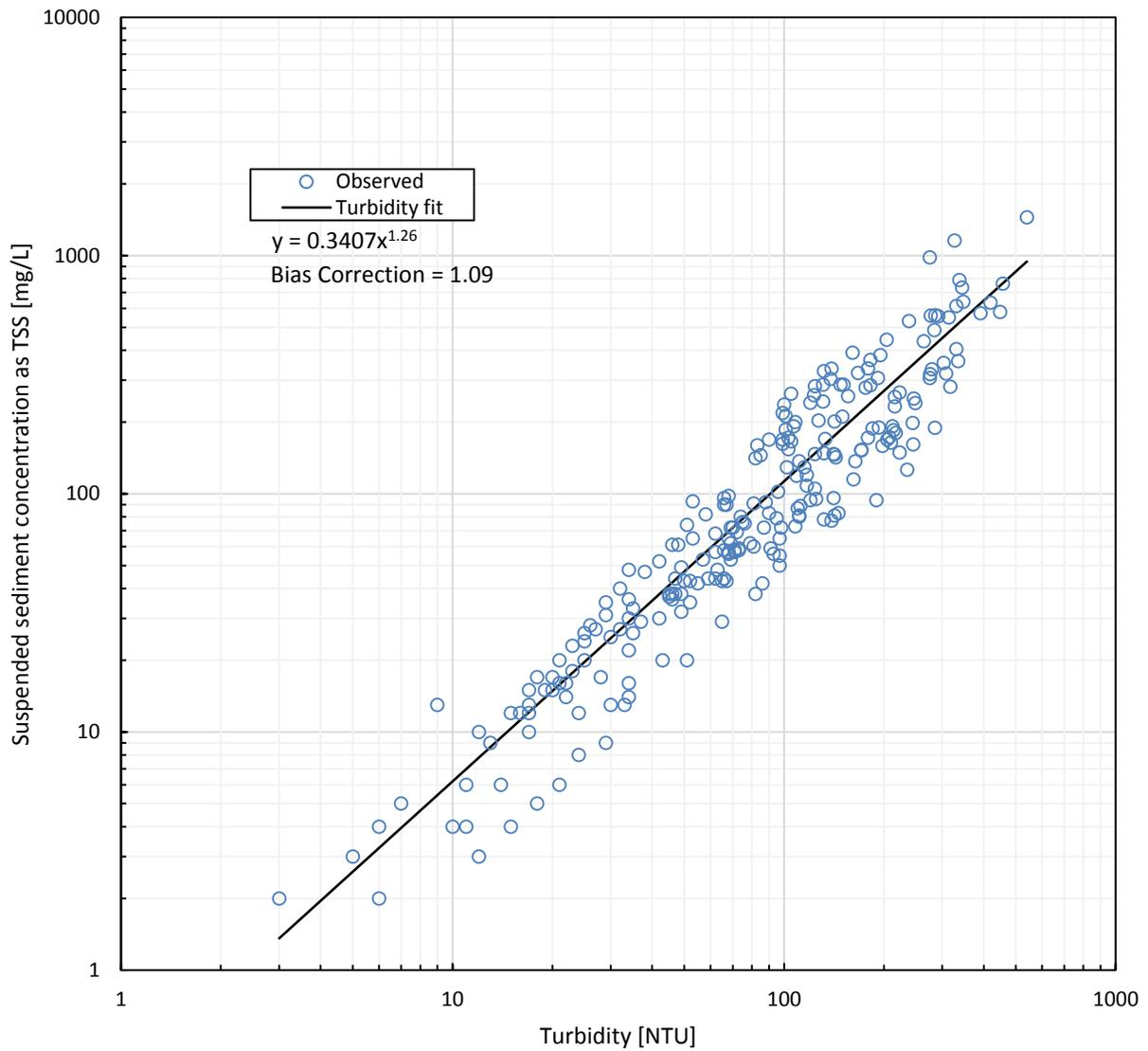
Figure 20. Rating curve for Sessom Creek suspended sediment (as TSS) concentration based on turbidity
