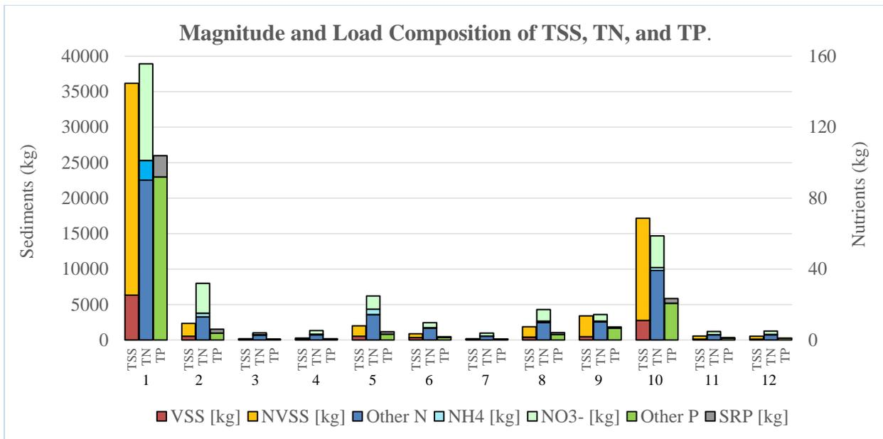
Figure 36. Load compositions during 12 storm events. “Other N” and “Other P” correspond to undifferentiated forms of TN and TP, most of which are assumed to be particulate organic or inorganic.
