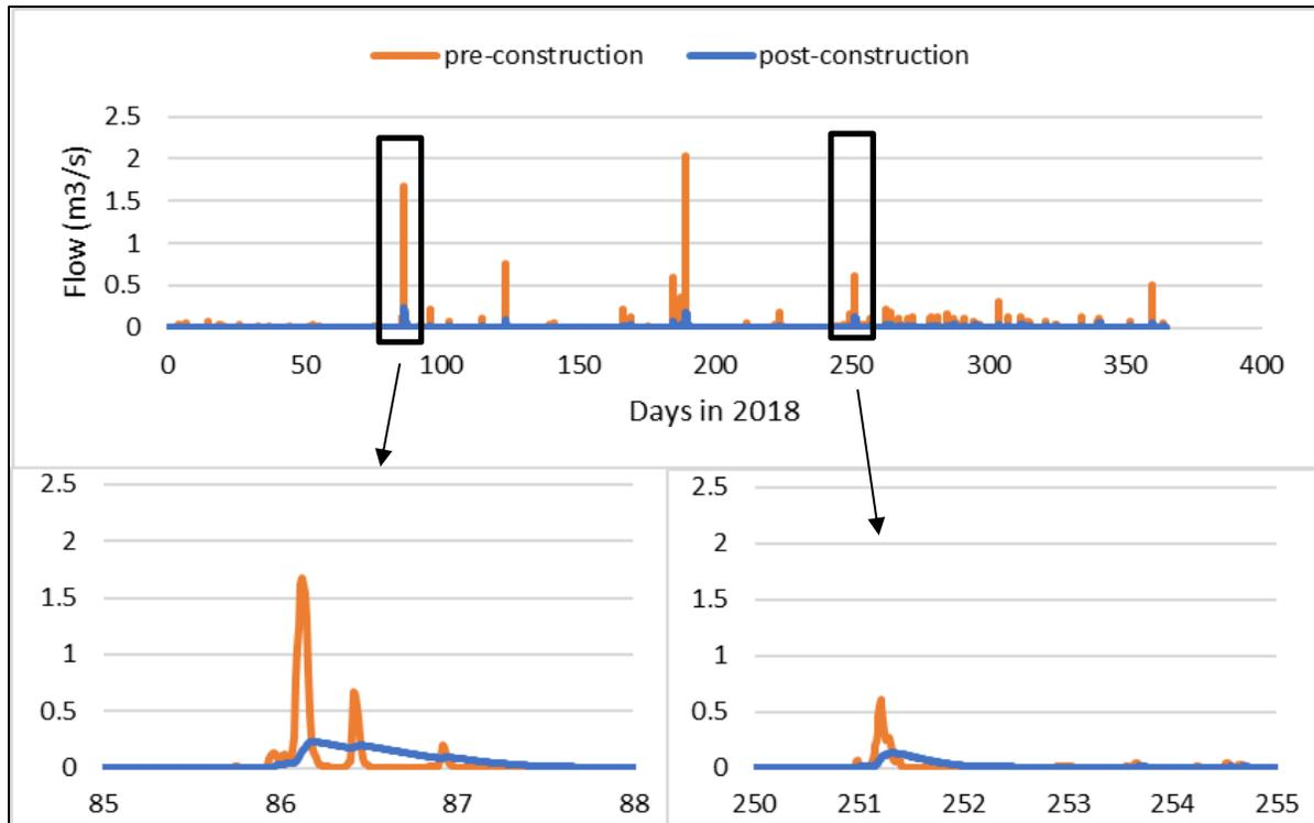
Figure 24. Modeled channel flow at the outlet of Windmill tributary comparing pre- and post-construction of a proposed detention pond.
