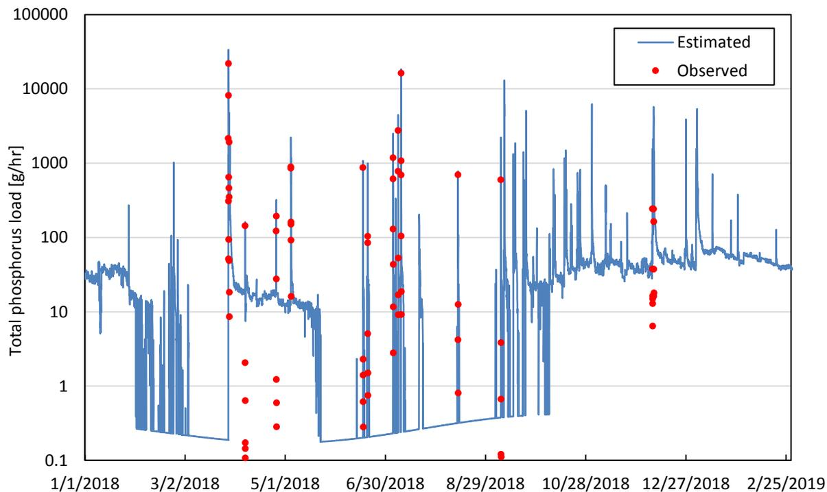
Figure 16. LOADEST estimated vs observed total phosphorus loads during the monitoring period 1 Jan 2018 to 28 February 2019.
