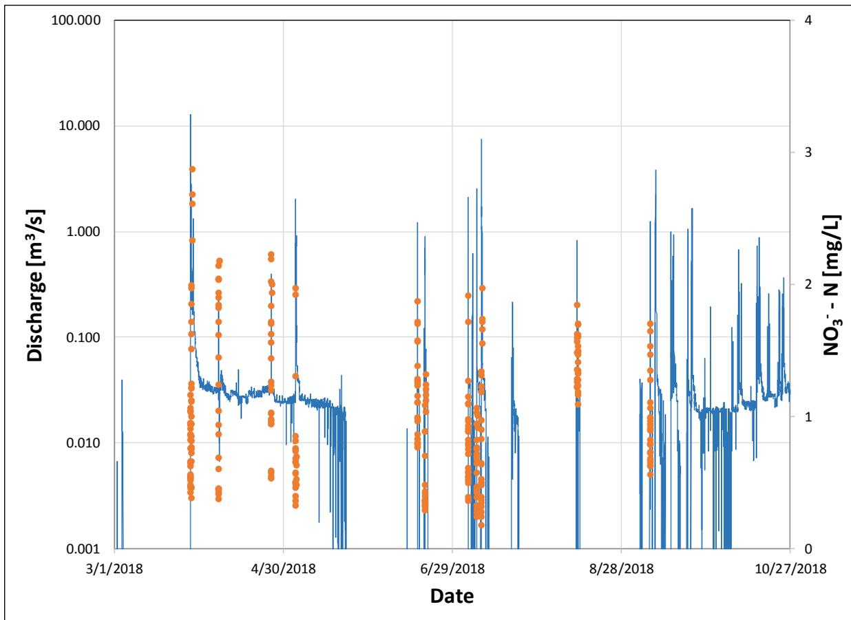
Figure 27. Nitrate as Nitrogen ( $\text{NO}_3^-$ -N) concentrations in stormwater samples. Note that the NPS axis is linear, while the discharge axis is logarithmic.
