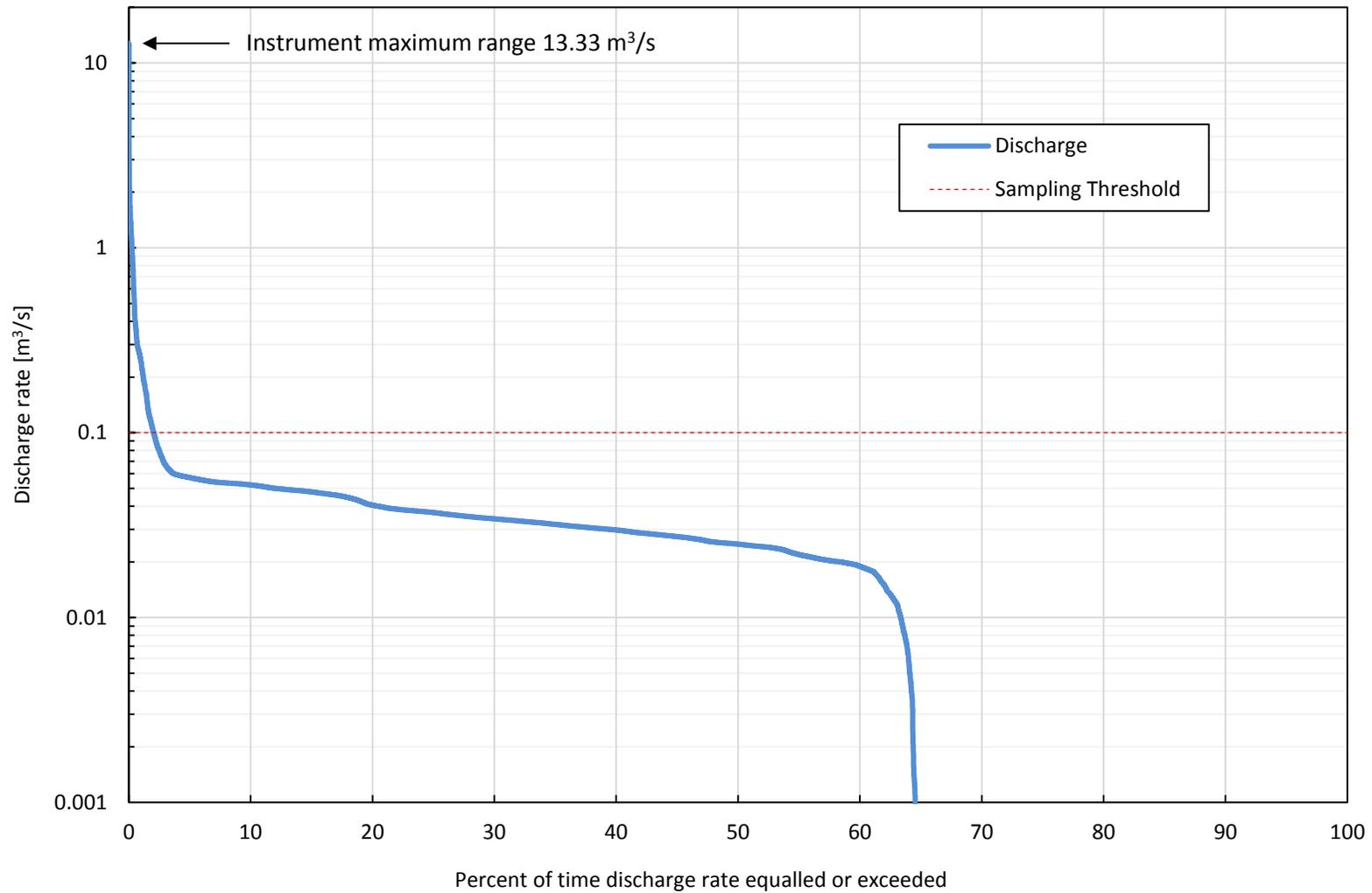
Figure 11. Sessom Creek flow duration curve. Curve based on continuous NOAA record between 1 January 2018 and 28 February 2019. Maximum discharge measurement 13.33 m<sup>3</sup>/s (instrument limitation) and minimum was 0.001 m<sup>3</sup>/s. Dotted red line indicates automated sampler activation threshold (0.1 m<sup>3</sup>/s) above which water quality samples were collected.
