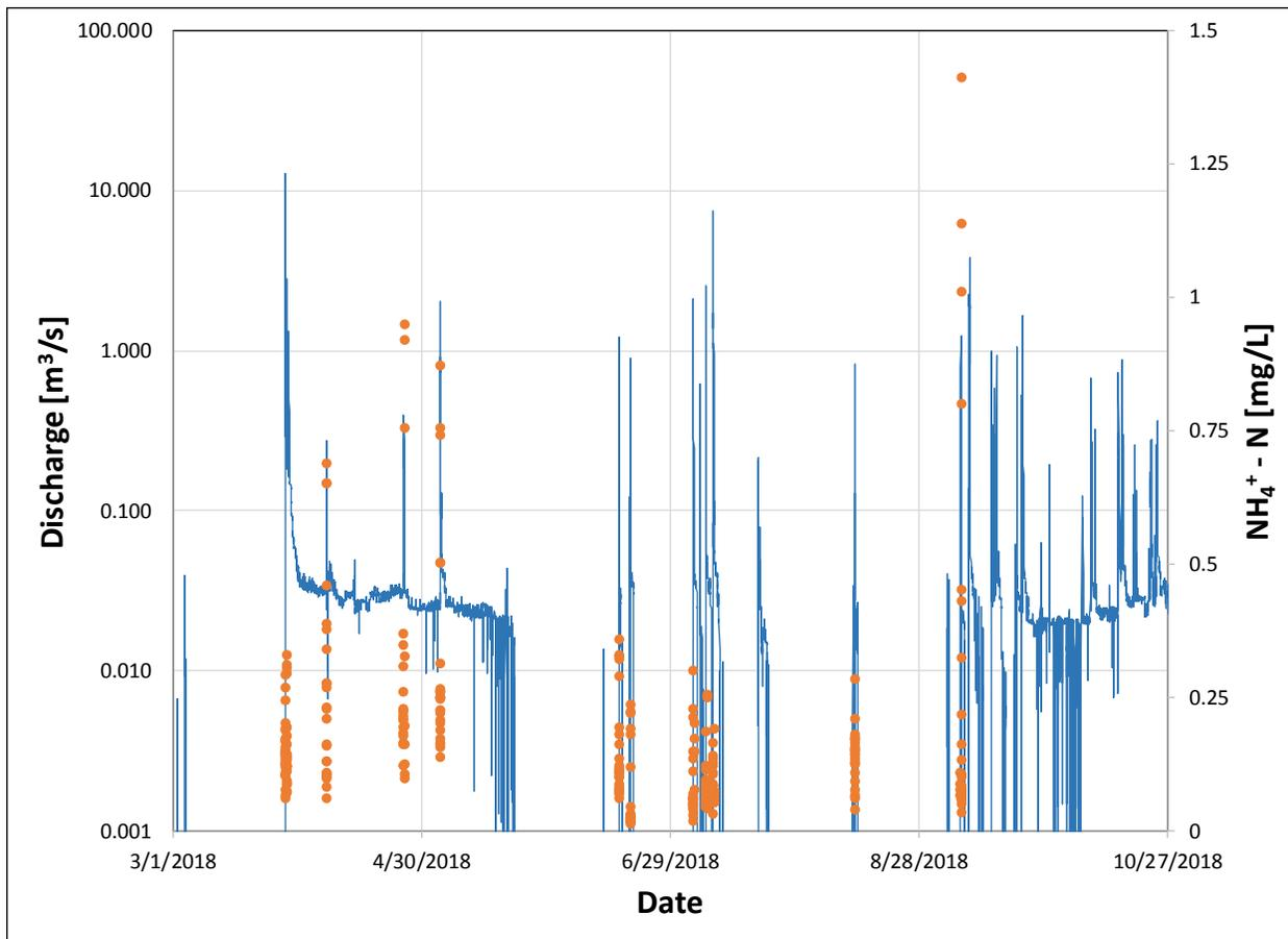
Figure 26. Ammonium as Nitrogen (NH<sub>4</sub><sup>+</sup>-N) concentrations in stormwater samples. Note that the NPS axis is linear, while the discharge axis is logarithmic.
