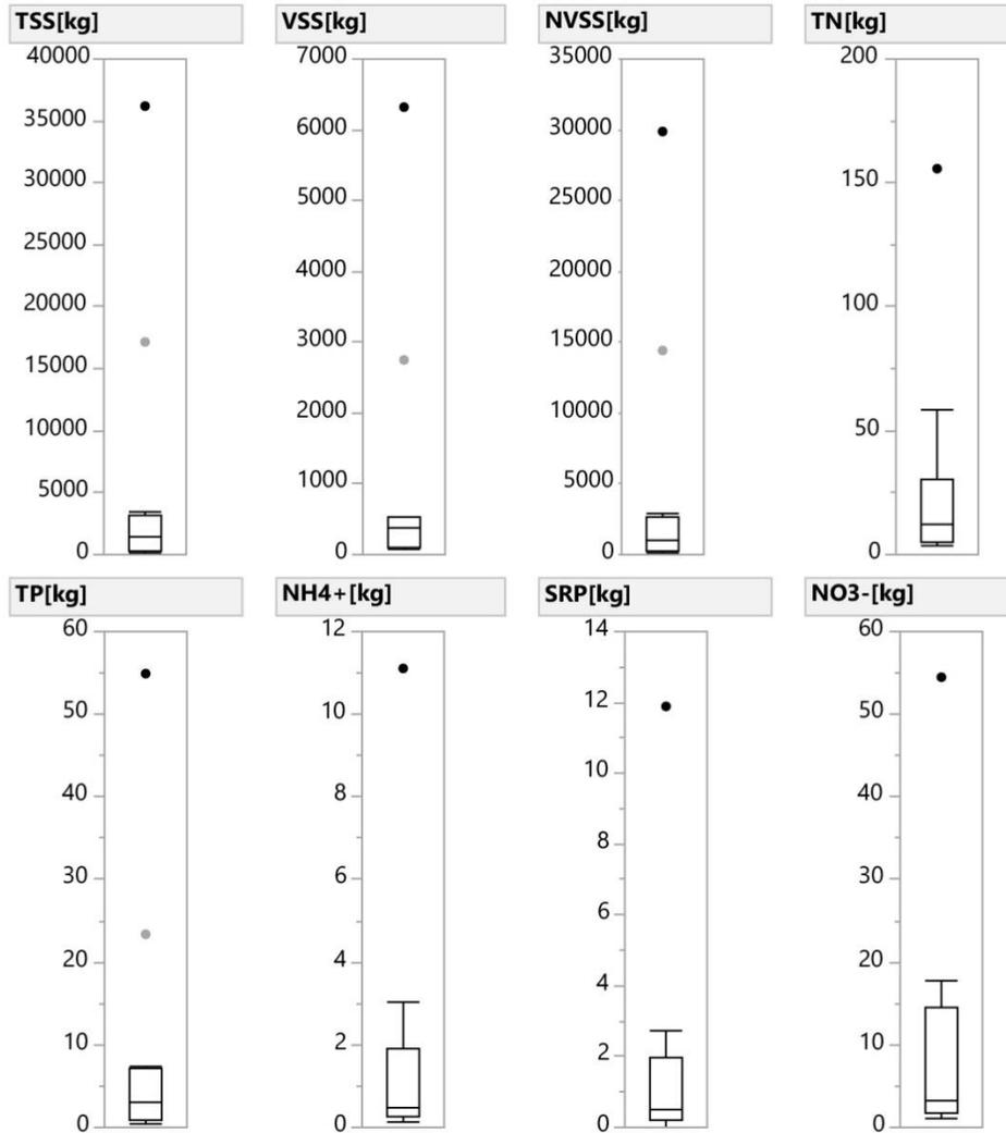
Figure 34. Box and whisker outlier plots for total loads of all 12 storm events. Note the two largest storm events (#1 and #10) that plot as statistical outliers for most parameters. Mean and quartiles are illustrated.
