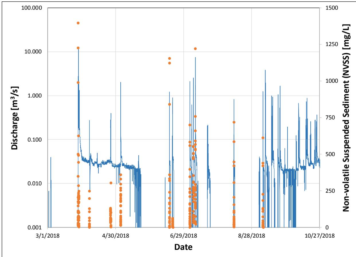
Figure 30. Non-volatile Suspended Sediments (VSS) concentrations in stormwater samples. NVSS is the inorganic portion of Total Suspended Sediments (TSS), and represents mineral grains and other non-organic sediments. Note that the NPS axis is linear, while the discharge axis is logarithmic.
