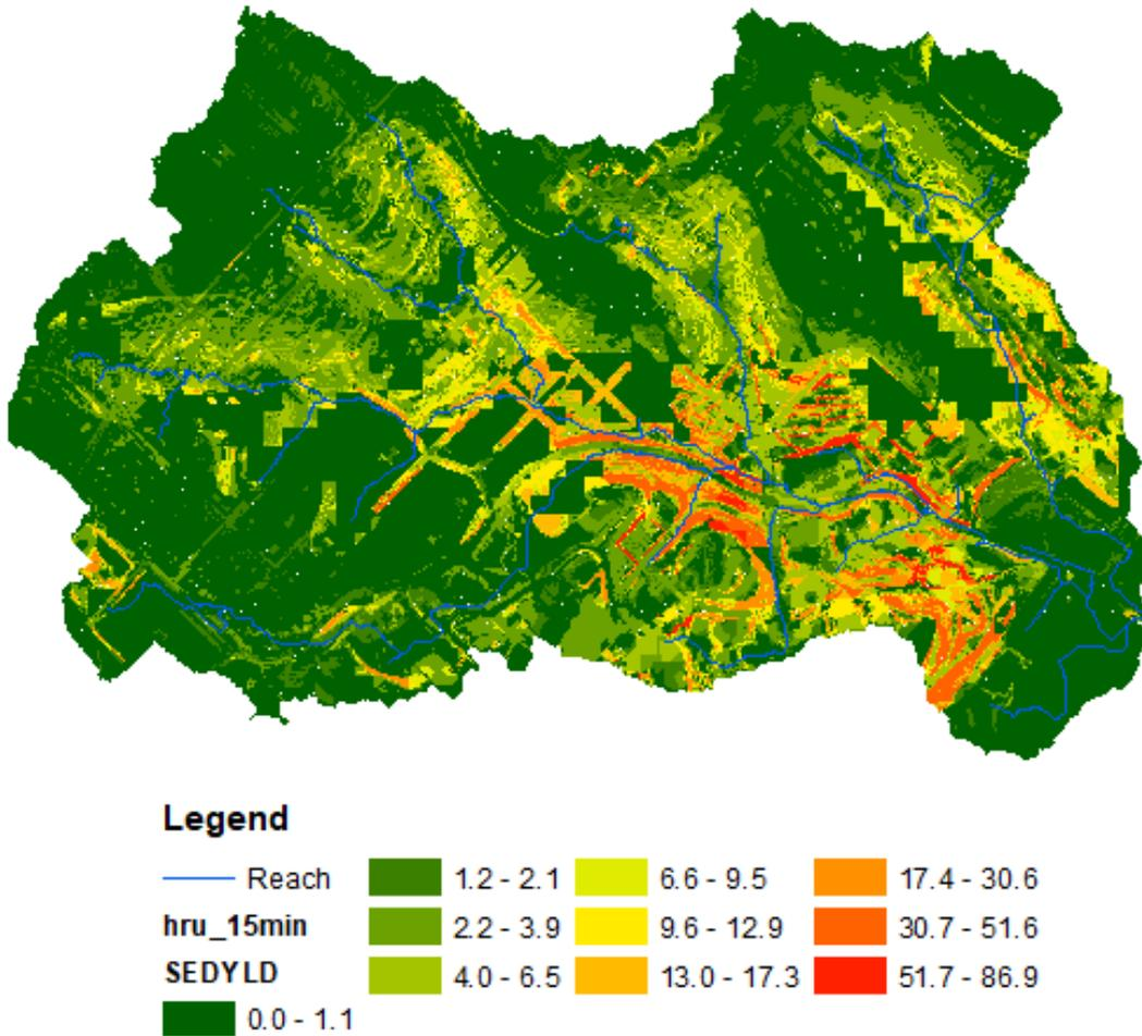
Figure 23. Modeled annual soil erosion rate by HRU (metric tons/ha).
