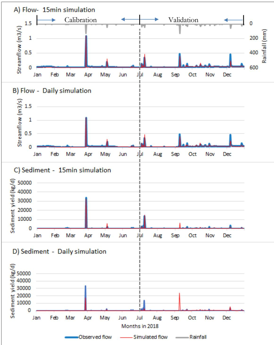
Figure 21. Calibrated daily flow and sediment yield from SWAT 15-min and daily interval models. 3A and 3C are simulated with 15-min interval and 3B and 3D are daily results.
