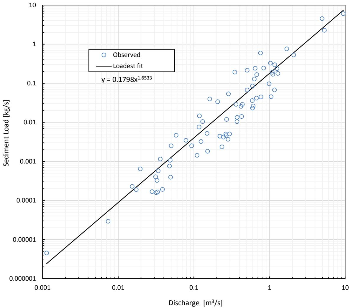
Figure 14. LOADEST rating curve for Sessom Creek sediment loads, measured as TSS. Assuming that this relationship remains unchanged in the future, estimated TSS loads may be calculated by using the above relationship and integrating across the discharge for a storm event.
