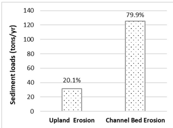
Figure 22. Origins of the sediment delivered to the watershed outlet.
