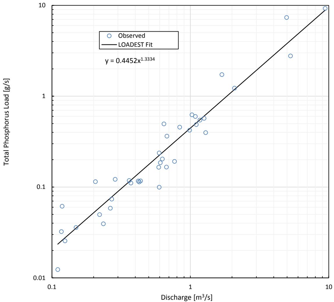
Figure 17. LOADEST rating curve for Sessom Creek total phosphorus loads. Assuming that this relationship remains unchanged in the future, estimated TP loads may be calculated by using the above relationship and integrating across the discharge for a storm event.
