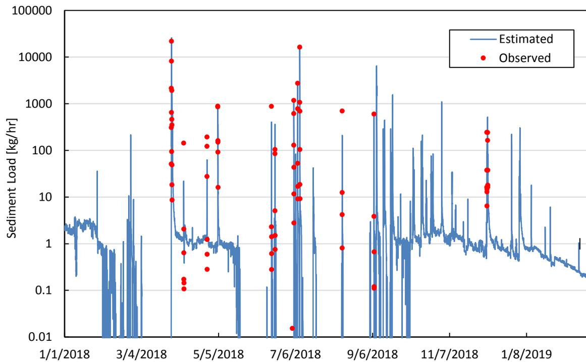
Figure 13. LOADEST estimated vs observed suspended sediment loads during the monitoring period 1 Jan 2018 to 28 February 2019.
