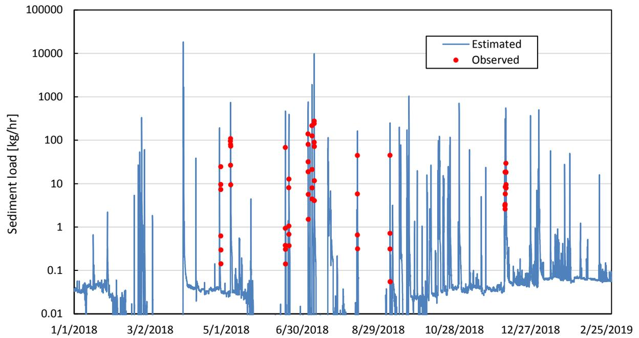
Figure 19. Sediment loads estimated by turbidity vs observed during the monitoring period 1 Jan 2018 to 28 February 2019.
