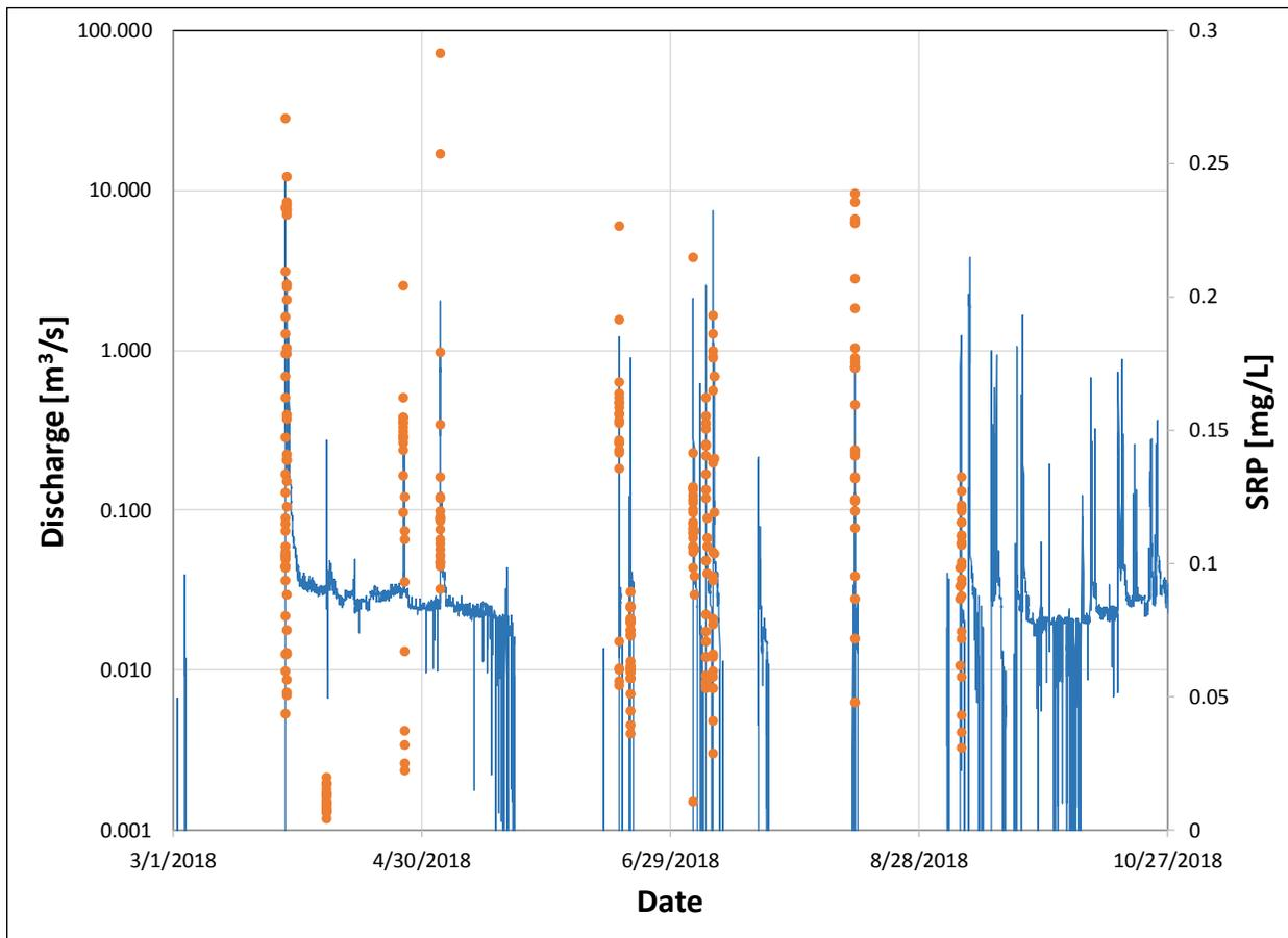
Figure 28. Soluble Reactive Phosphorous (SRP) concentrations in stormwater samples. Note that the NPS axis is linear, while the discharge axis is logarithmic.
