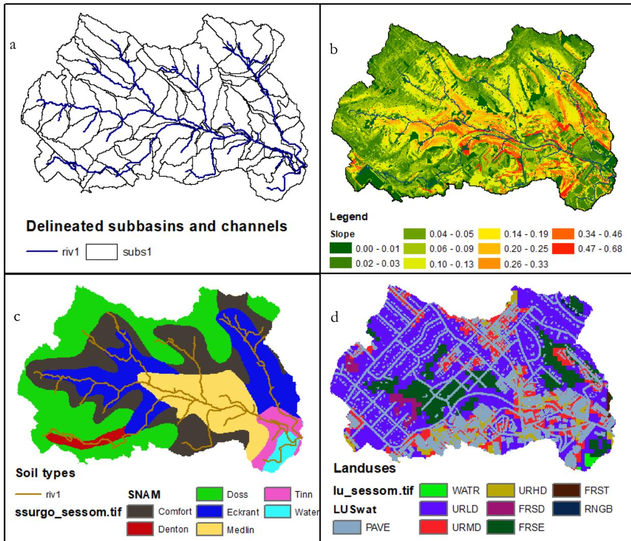
Figure 9. SWAT input data layers. a: main channels and sub-basins, b: land slope, c: soil names, d: land use types.
