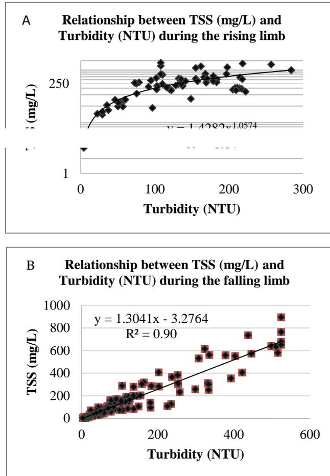
Figure 33 Relationship between TSS and Turbidity during the rising (A) and falling limb (B) of the hydrograph.
