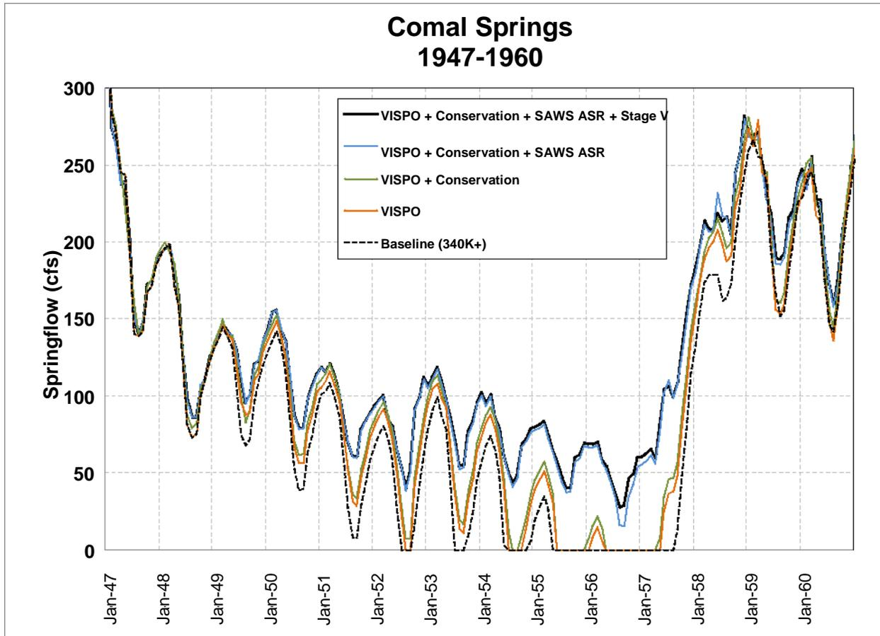
**Figure 5-4:** Simulated Monthly Average Springflow at Comal Springs (1947-1960)
