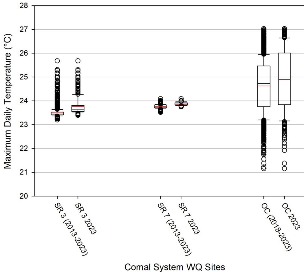
Figure 3.1-12. Box plots of maximum water daily temperatures (°C) among Comal system RTWQ sites from time of deployment through 2023 compared to 2023. Black lines represent median values and red lines denote mean values. Whiskers represent maximum and minimum temperature values, excluding outliers (open circles).
