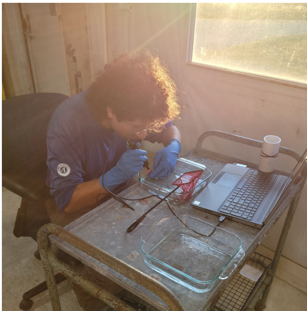
Figure 2. Kevin Rubio (SCA) scanning salamanders tagged with p-Chips and serving as a novice reader.
