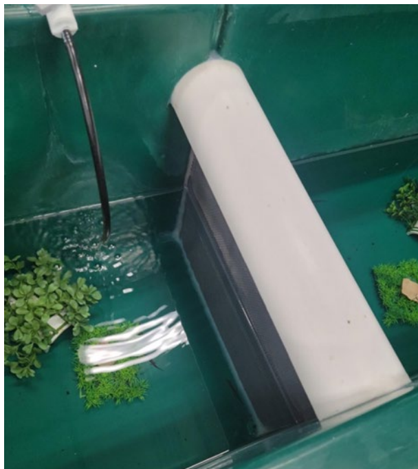
Figure 1. A PVC pipe cut in half is placed on tank dividers to prevent salamanders from moving between sections.
