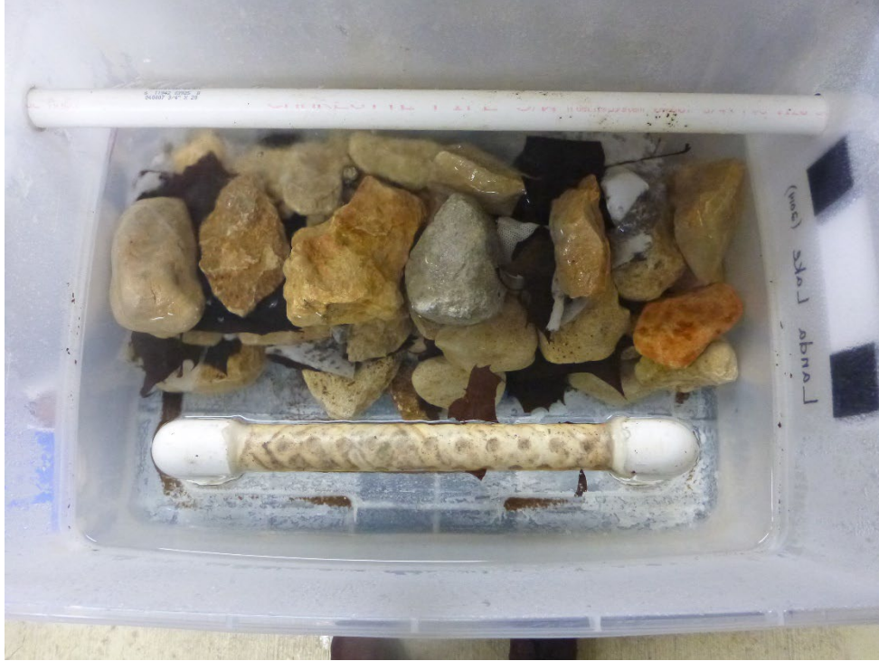
Figure 5 Easy-Upwelling system (Huston and Gibson 2015) utilizes stacked limestone rocks, conditioned leaves, and conditioned cloth as CSR habitat. Water enters from PVC spray bar (1/16" equidistant holes drilled lengthwise) and exits through a PVC outflow pipe wrapped in 200-220 \mu m mesh screen.
