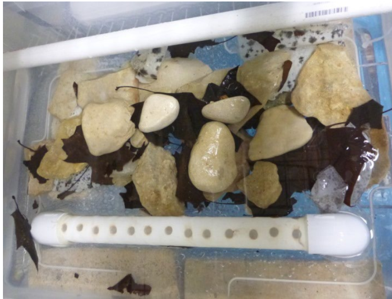
Figure 7. Height of stacked limestone, leaf, and cloth substrate was reduced and spread out further.
