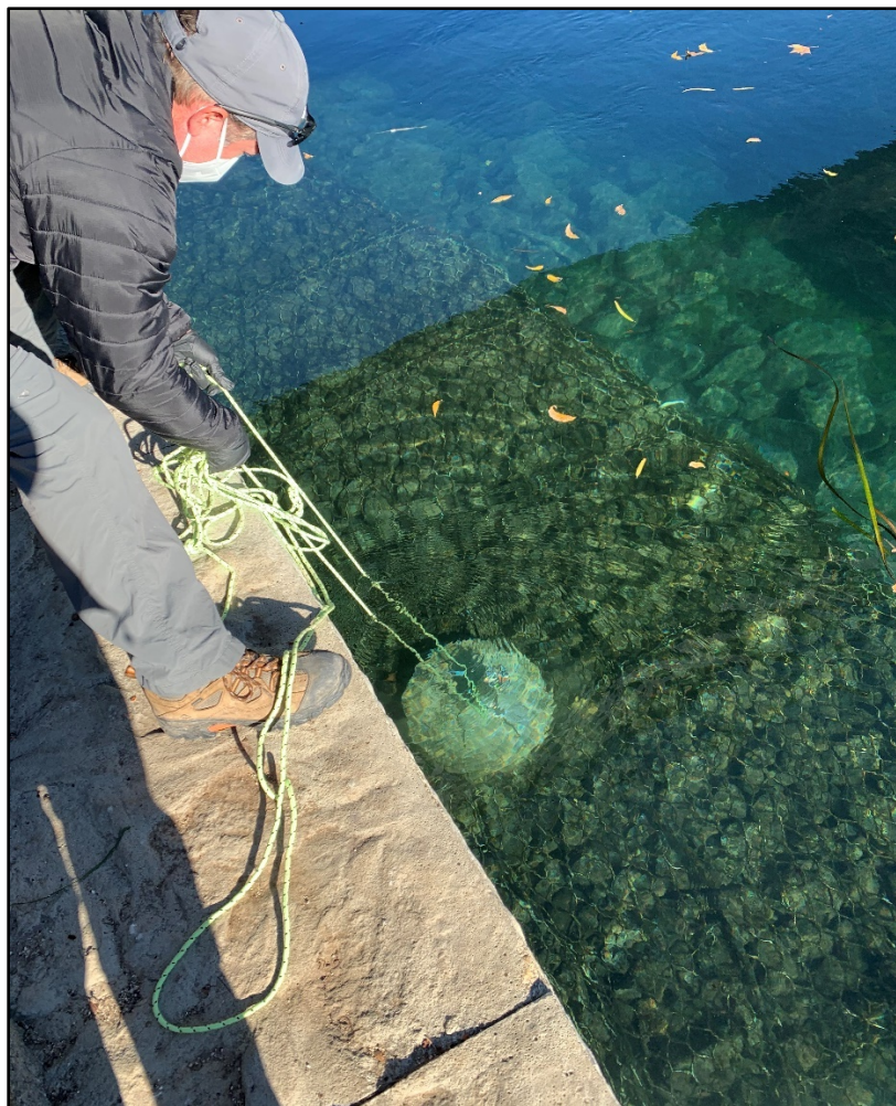
Figure 3. Passive Diffusion Sampler (PDS) Installation at Sample Location HCS430
