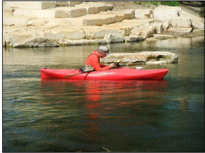
Kayak-mounted GPS equipment used during aquatic vegetation mapping.
