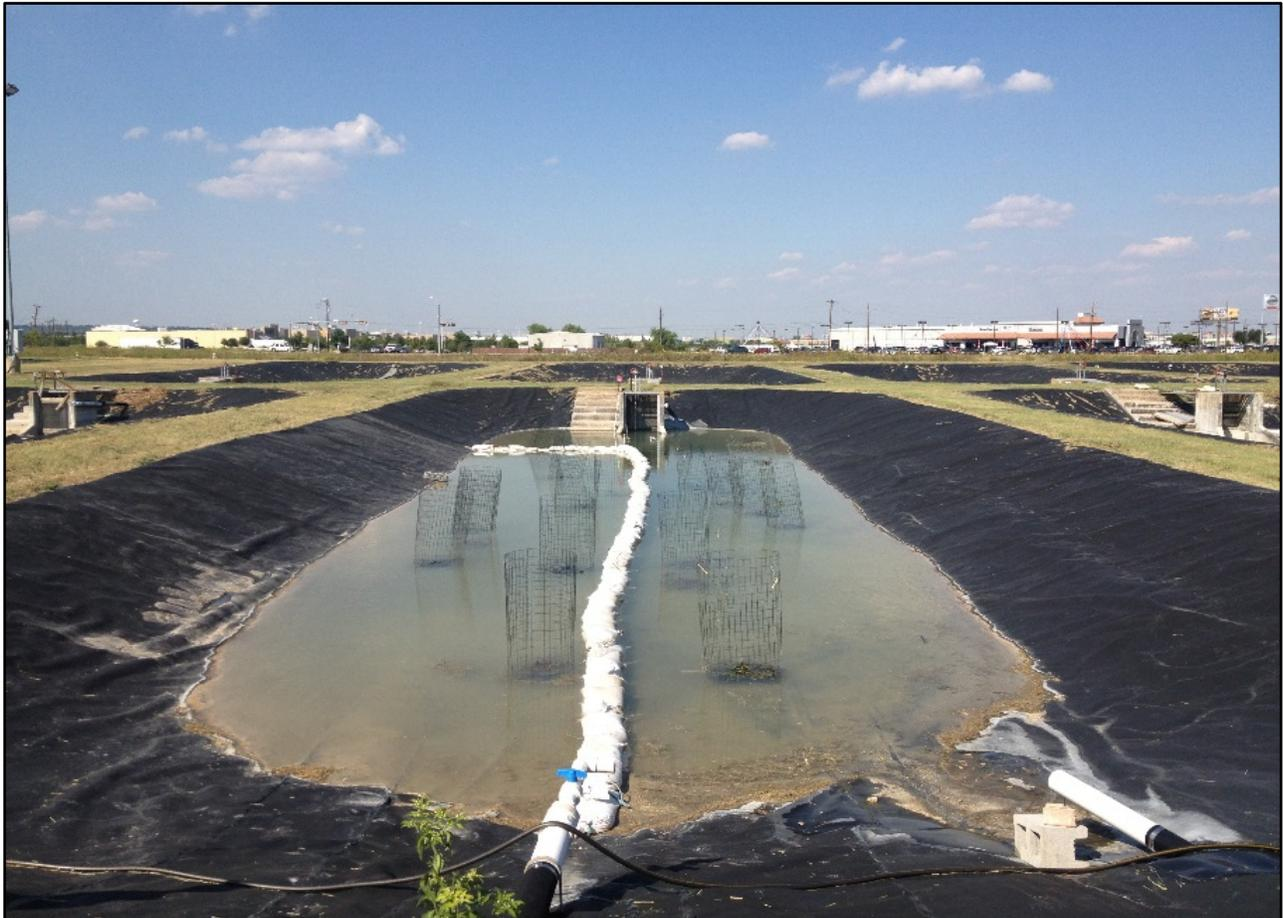
**Figure 33.** Division of the experimental pond into two treatment areas. The flowing treatment is on the right, the inlet pipe providing fresh water can be seen in the lower right.
