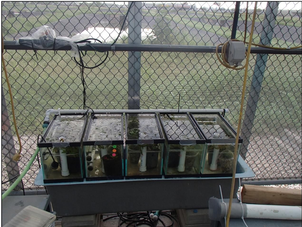
**Figure 18.** Pre-trial 1 equipment setup, including a five-tank array plumbed with various CO<sub>2</sub> concentration and water temperature treatments.
