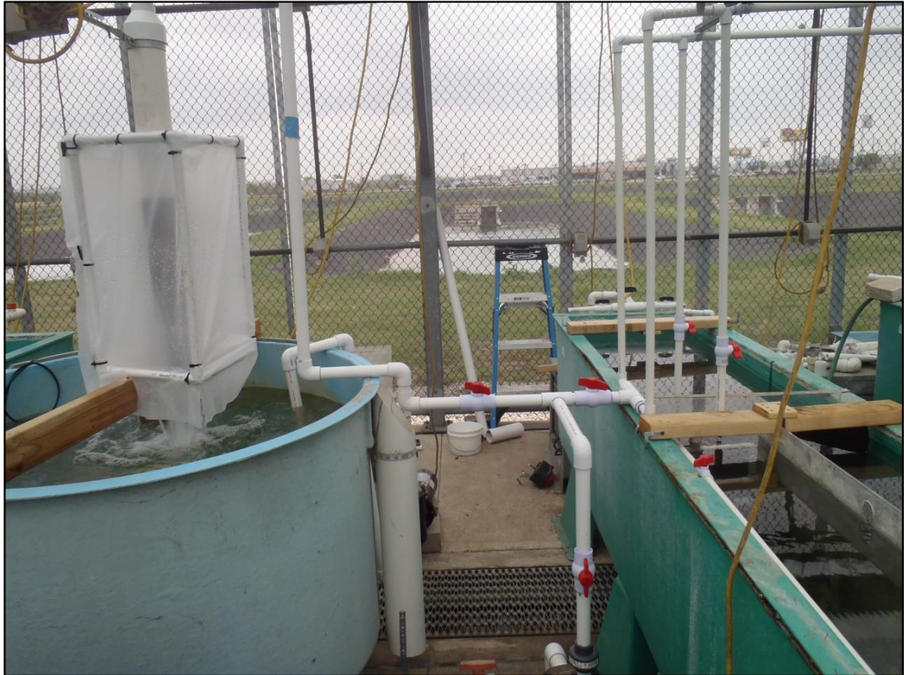
**Figure 3. Reservoir Tank with CO<sub>2</sub> degasser (left) and living stream divided in two right).**
