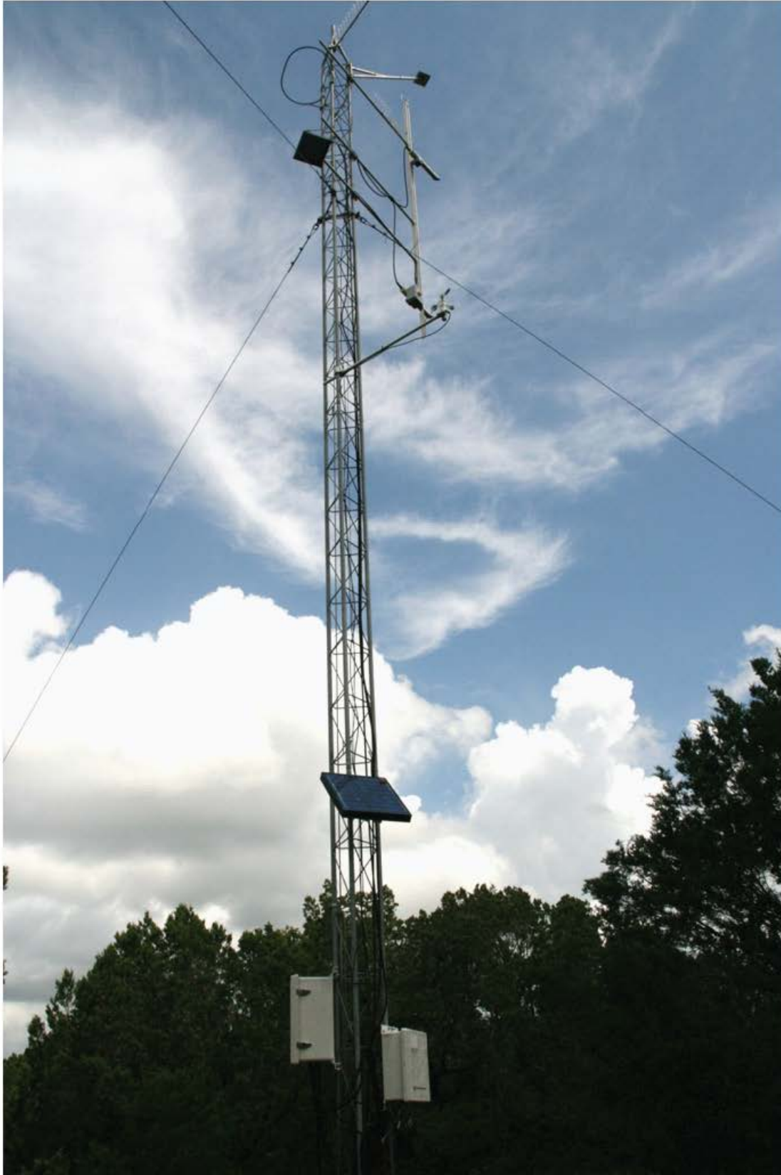
Figure 4. Evapotranspiration station in the reference watershed at site RWS_{ET} (U.S. Geological Survey station 295104098285900 Honey Creek reference evapotranspiration near Spring Branch, Texas), Honey Creek State Natural Area, Comal County, Tex., July 23, 2010.
