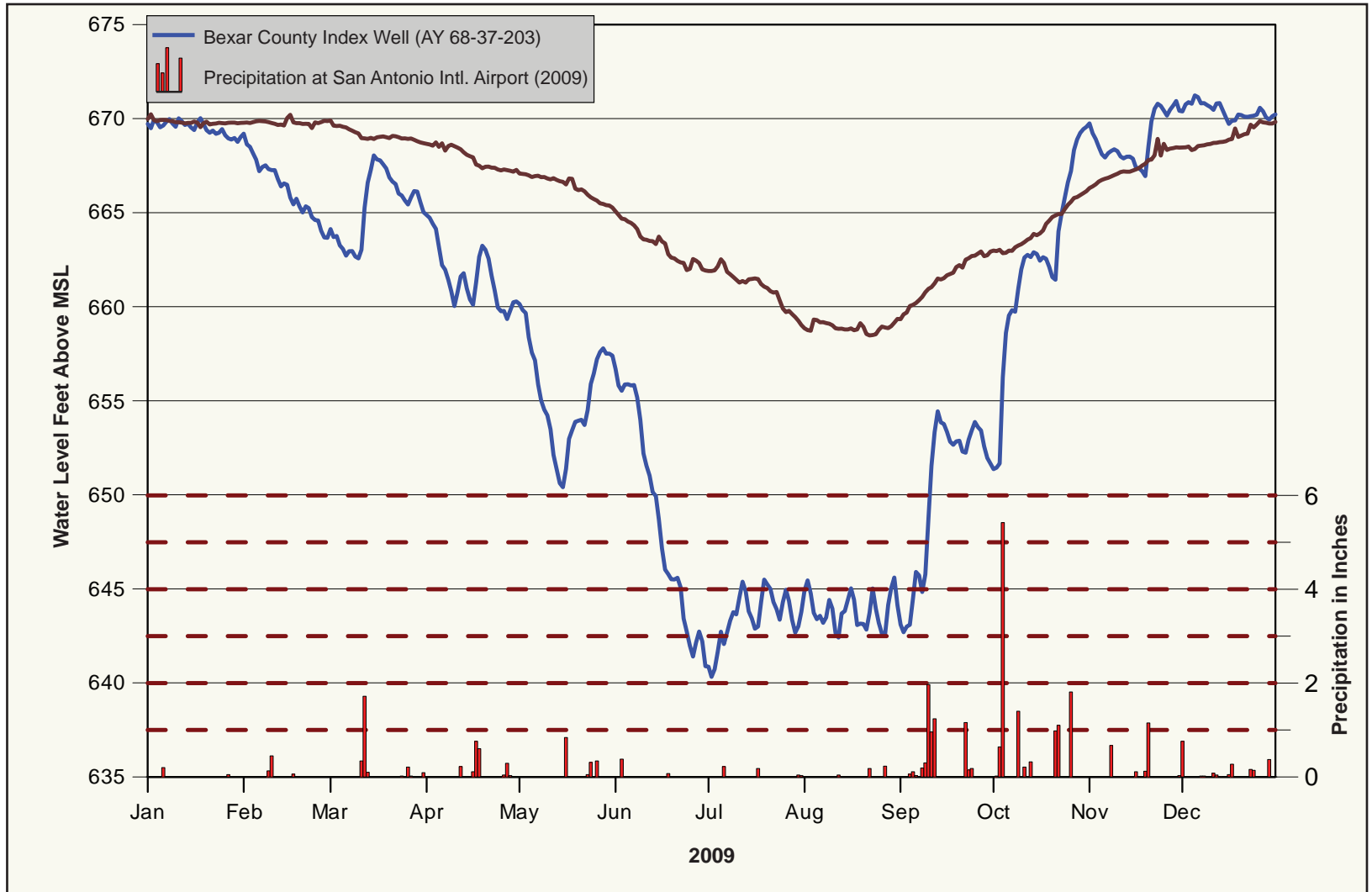
Figure B-1. Bexar County Index Well J-17 (AY-68-37-203) Hydrograph of Groundwater Elevation vs. Precipitation at San Antonio International Airport
